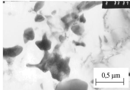
Fig. 22. The substructure of HCM12A steel with Laves phases
