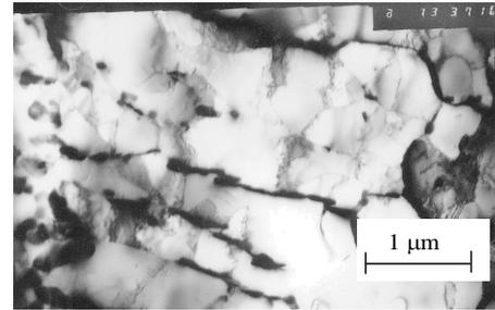
Fig. 16. Subgrain structure with intensive effect of precipitation of carbides and the occurrence of recovery processes in the matrix
