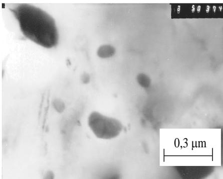
Fig. 21 a. The substructure of HCM12A steel with  $M_{23}C_6$  and MX carbides. Details from Fig. 20
