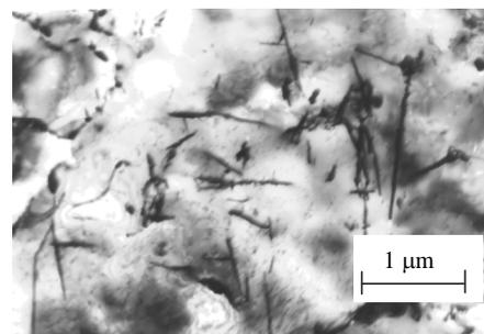
Fig. 5.  $\delta$ -Ferrite with acicular precipitations of  $M_{23}C_6$
