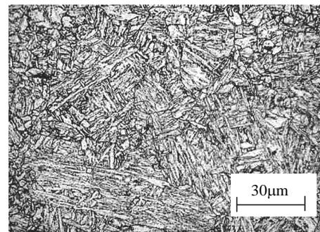
Fig. 18. HCM12A steel microstructure after 30 thousand hours of operation. LM
