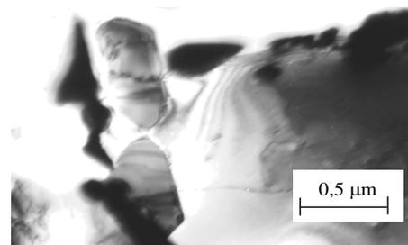
Fig. 12.  $M_{23}C_6$  carbide precipitations in the HCM12A steel (bright field)
