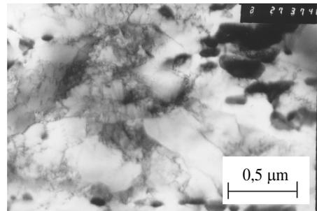
Fig. 24. The recovery processes in the matrix of HCM12A steel after 30<sup>th</sup> hours of operation
