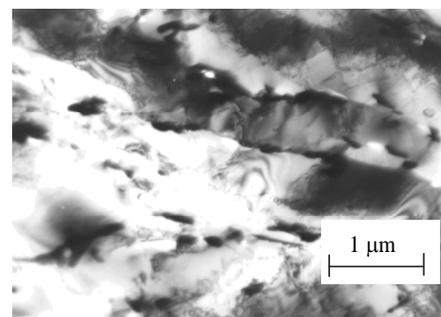
Fig. 6. Tempered martensite laths with  $M_{23}C_6$  carbide precipitations of on grain boundaries
