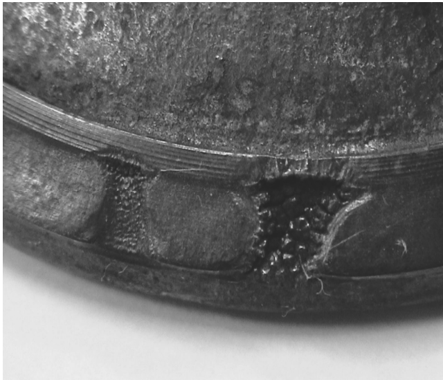
Fig. 1. An example of valve failure during the service
