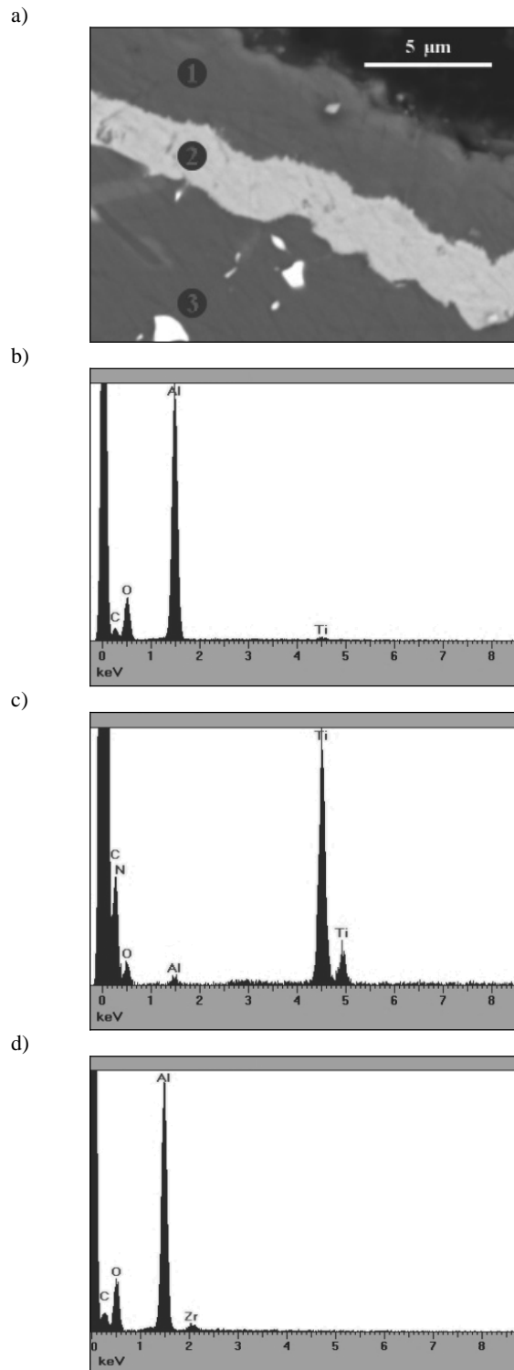
Fig. 14. a) Fracture surface of the TiN+Al 2 O 3 coating deposited on Al 2 O 3 +ZrO 2 substrate, b) X-ray energy dispersive plot the area 1 as in figure a, c) X-ray energy dispersive plot the area 2 as in figure a, d) X-ray energy dispersive plot the area 3 as in figure a.
