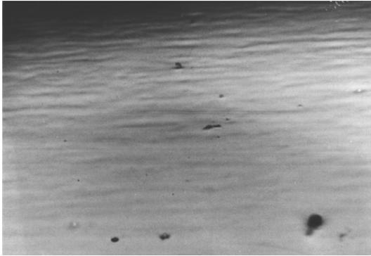
Fig. 3. The surface fractography of the surface of as received sample before the corrosion test, magnitude 200x
