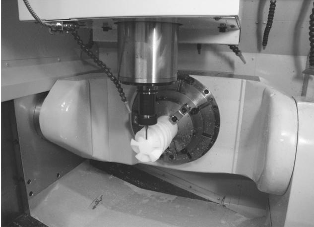
Fig. 10. The four-axis machining of model material on five-axis machine tool
