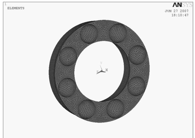
Fig. 2. The finite element model of bearings
