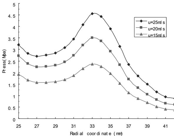
Fig. 4. The pressure distribution of diametrical direction
