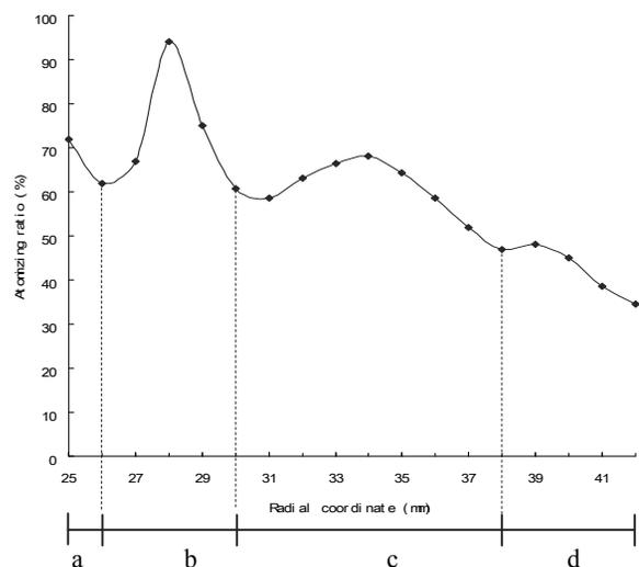
Fig. 5. The atomizing ratio distribution of the spraying oil
