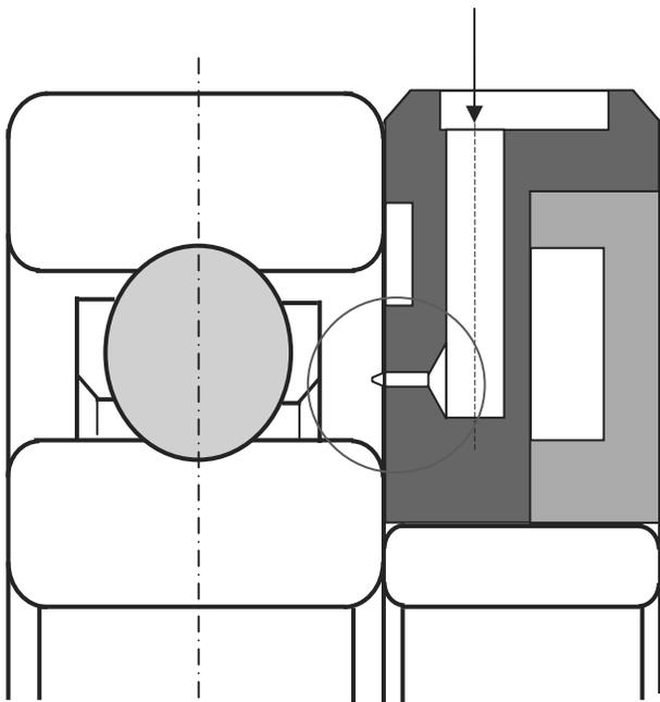
Fig. 1. Diagrammatic Sketch of the oil supply system
