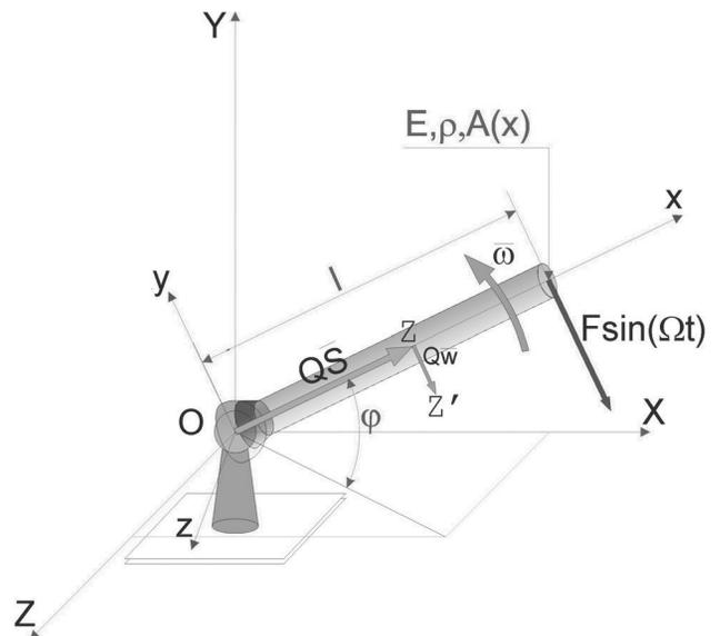
Fig. 5. The model of fixed beam in transportation
