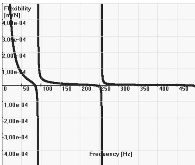
Fig. 6. The dynamical flexibility (18) of stationary free-free beam
