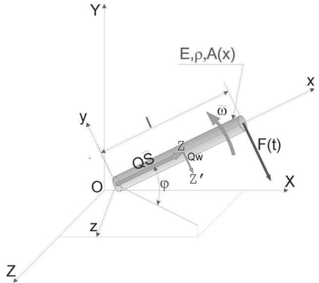
Fig. 4. The model of free-free beam in rotation
