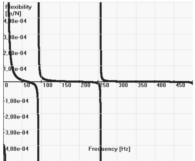
Fig. 7. The dynamical flexibility (18) of stationary free-free beam
