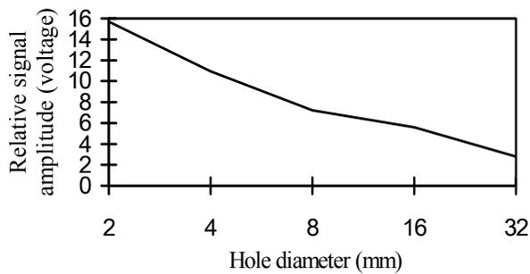
Fig. 15. Relationship between signal amplitude and 75 × 100mm simulator for water and 1 MHz frequency
