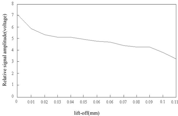
Fig. 4. Signal amplitude of sender fixed and receiver lift-off for 1MHz
