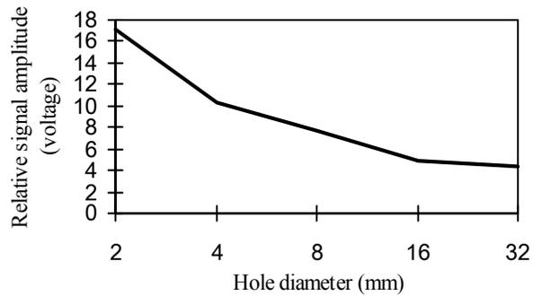
Fig. 17. Relationship between signal amplitude and 75 × 75mm simulator for viscous fluid and 1 MHz frequency
