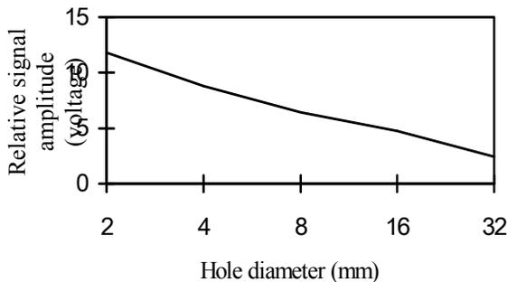
Fig. 8. Relationship between signal amplitude and 75 × 75 mm simulator for air and 0.6 MHz frequency
