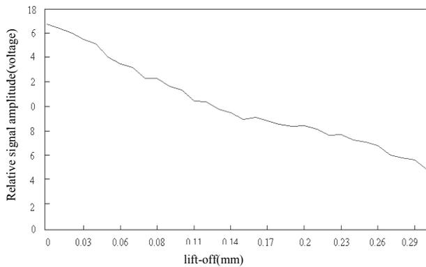
Fig. 5. Signal amplitude of receiver fixed and sender lift-off for 1MHz
