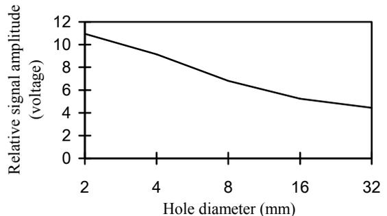
Fig. 12. Relationship between signal amplitude and 75 × 75mm simulator for water and 0.6 MHz frequency
