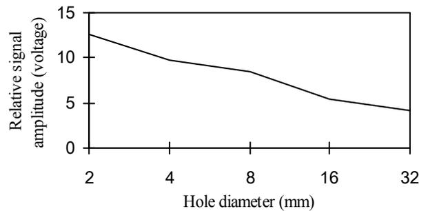
Fig. 18. Relationship between signal amplitude and 75 × 100mm simulator for viscous fluid and 0.6 MHz frequency
