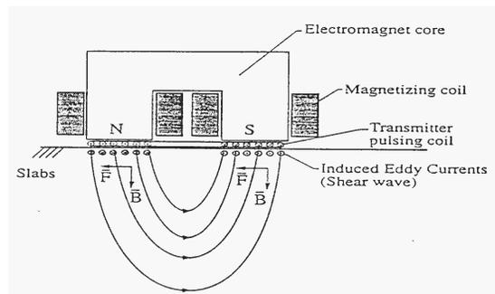
Fig. 1. Basic principle of EMAT echo sensor
