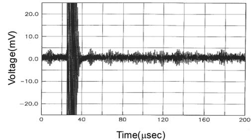
Fig. 6. Ultrasonic wave response according to a change of hole size
