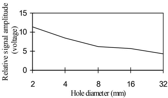
Fig. 13. Relationship between signal amplitude and 75 × 75mm simulator for water and 1 MHz frequency
