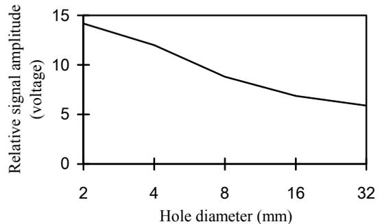
Fig. 11. Relationship between signal amplitude and 75 × 100 mm simulator for air and 1 MHz frequency
