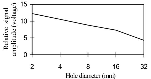
Fig. 19. Relationship between signal amplitude and 75 × 100mm simulator for viscous fluid and 0.6 MHz frequency
