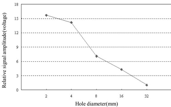
Fig. 7. Relation between the signal amplitude and hole diameter
