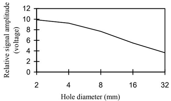
Fig. 10. Relationship between signal amplitude and 75 × 100 mm simulator for air and 0.6 MHz frequency
