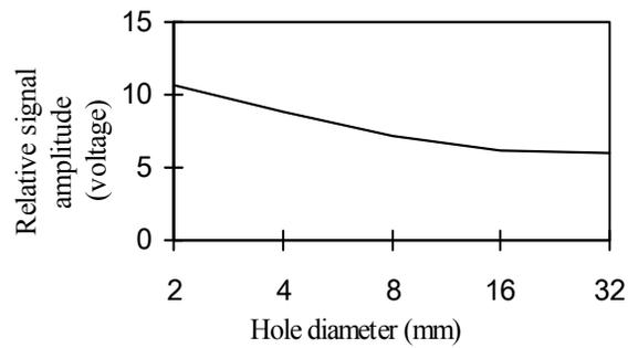
Fig. 9. Relationship between signal amplitude and 75 × 75 mm simulator for air and 1 MHz frequency
