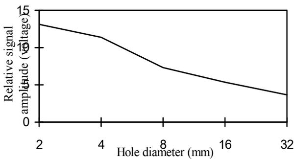
Fig. 14. Relationship between signal amplitude and 75 × 100mm simulator for water and 0.6 MHz frequency
