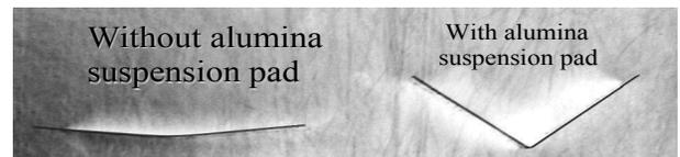
Fig. 8. V-bending samples. The left one is a sample of partial bending without the alumina suspension pad (air bending), and the right one is with it
