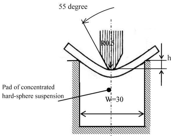
Fig. 7. Employed die and alumina concentrated hard-sphere suspension pad
