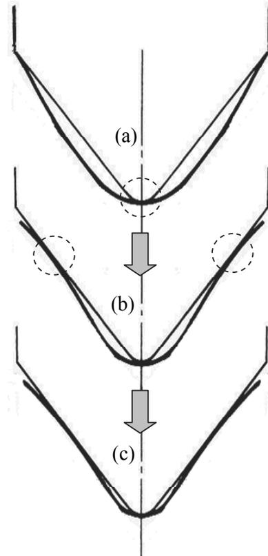
Fig. 13. Bending process with the suspension pad
