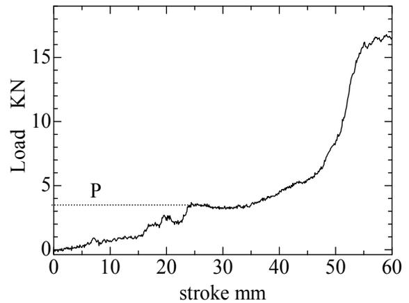
Fig. 4. Load change in backward extrusion test ( $\phi 2R=8$ , punch speed:1mm/s)
