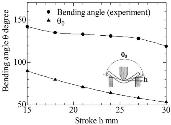
Fig. 10. Bending angle in partial bending (air bending)
