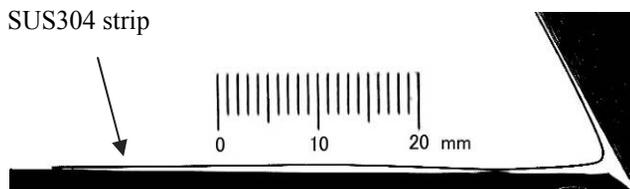
Fig. 12. Photograph of profile of a bent strip ( $h=24\text{mm}$ )
