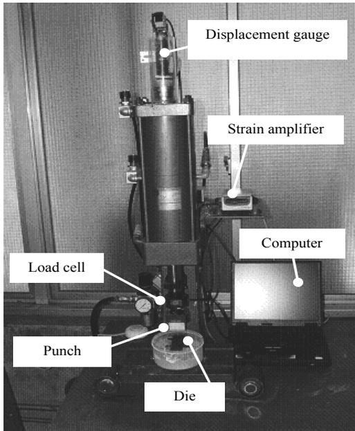
Fig. 6. Equipment for V bending experiment
