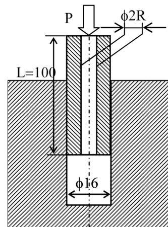
Fig. 3. Backward extrusion test
