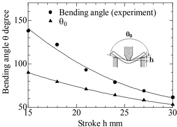
Fig. 11. Bending angle with alumina concentrated hard-sphere suspension pad
