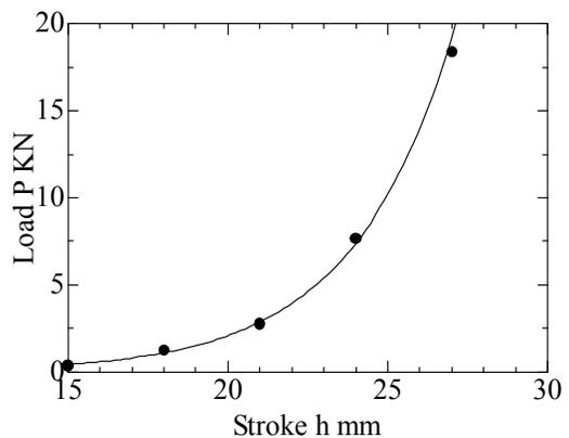
Fig. 9. Punch stroke and forming load
