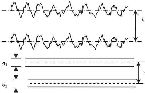
Fig. 4. a) Oil film thickness between the surfaces, b) Oil film thickness based on composite roughness
