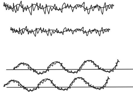
Fig. 7. a) Waviness or out-of-roundness smaller than roughness, b) Waviness or out-of-roundness larger than roughness
