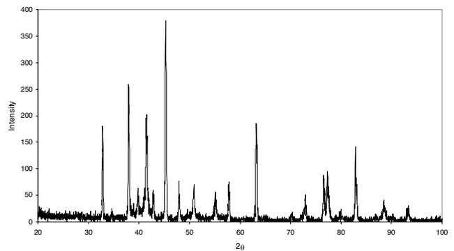
Fig. 5. XRD results for 1223 K, 6 hour borided AISI 1010 steel
