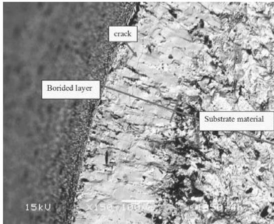
Fig. 9. Fracture surface of 1323 K, 4 h, borided specimen
