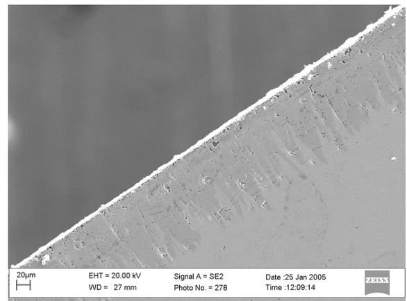
Fig. 6. SEM photograph of borided material at 1223°C for 4 hours, x200
