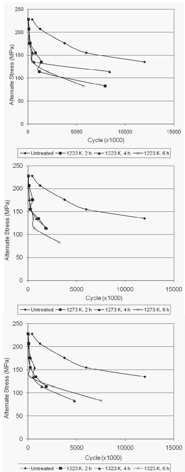
Fig. 8. S-N curves of borided AISI 1010 steel
