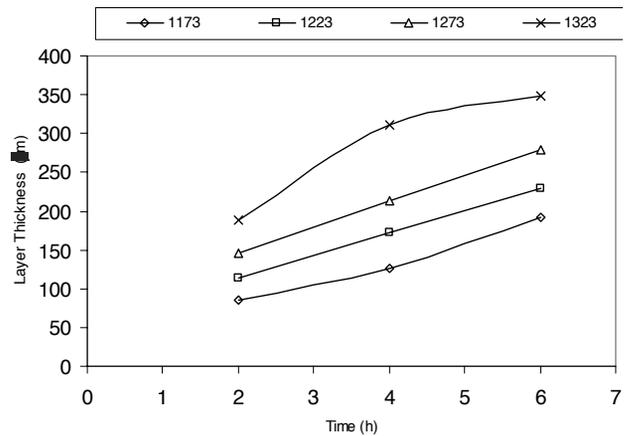
Fig. 4. Change of boride layer thickness
