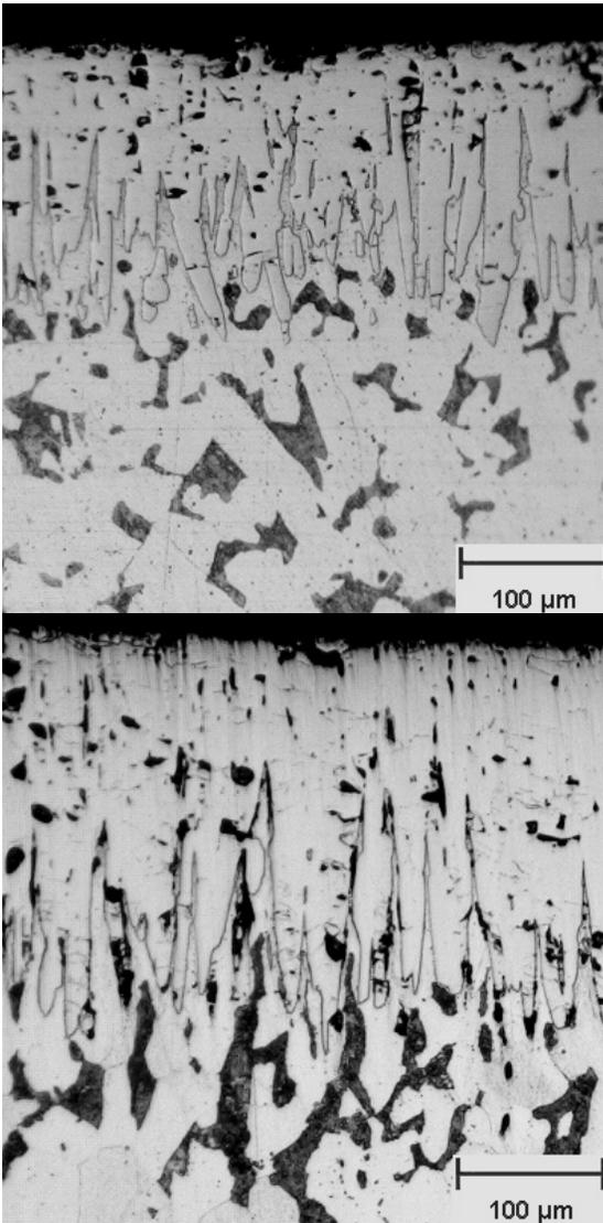
Fig. 3. Microstructure photograph of the material borided at 1173-1223-1273-1323 K temperatures for 4 hours, 100x, 5% Nital
