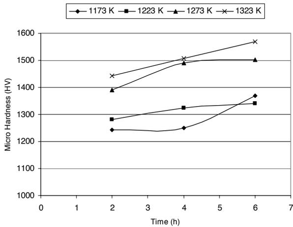
Fig. 7. Microhardness change depending on temperature and time
