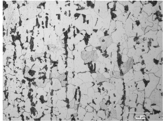
Fig. 2. Microstructure photograph of AISI 1010 steel 200x, %5 Nital
