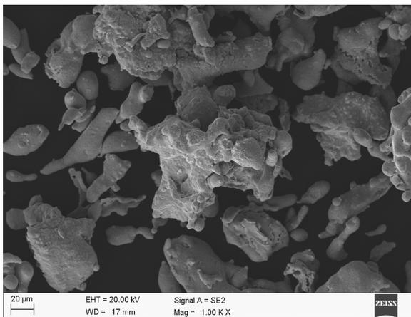
Fig. 1. Powder of high speed-steel M2 type atomized by water
