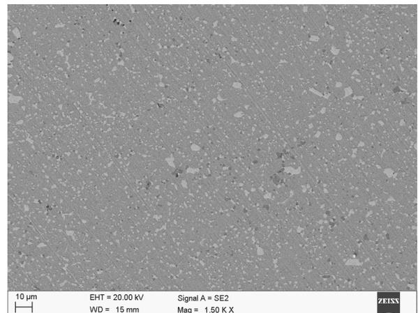
Fig. 10. Microstructure of M2, sintered under  $N_2$ -10% $H_2$  at 1260°C
