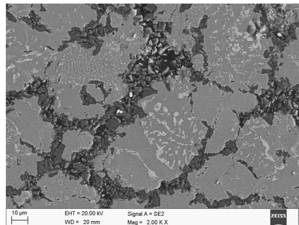
Fig. 6. Microstructure of M2 reinforced by TiC, sintered under vacuum at 1260°C
