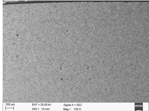
Fig. 5. Microstructure of M2/TiC graded material sintered, under N<sub>2</sub>-10%H<sub>2</sub> at 1260°C
