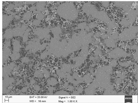
Fig. 12. Microstructure of M2 reinforced by TiC, sintered under N<sub>2</sub>-10%H<sub>2</sub> at 1310°C
