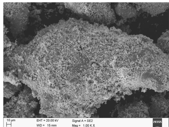
Fig. 4. Mixture of M2 and WC powders
