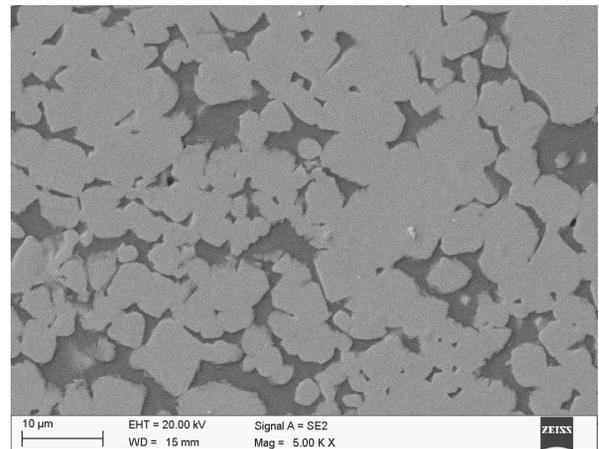
Fig. 9. Microstructure of M2 reinforced by WC, sintered under  $N_2$ -10% $H_2$  at 1260°C
