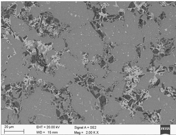
Fig. 7. Microstructure of M2 reinforced by TiC, sintered under  $N_2$ -10% $H_2$  at 1260°C
