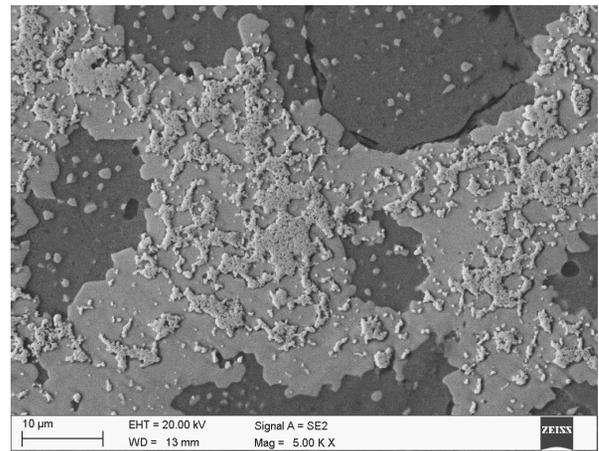
Fig. 8. Microstructure of M2 reinforced by WC, sintered under  $N_2$ -10% $H_2$  at 1210°C
