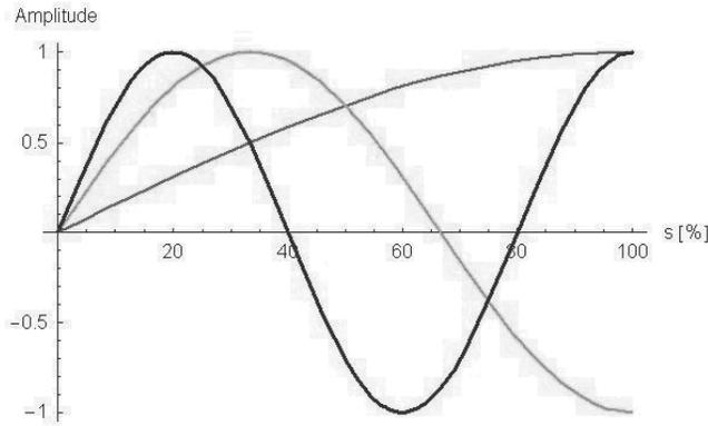
Fig. 5. The juxtaposition of first three forms of vibrations for the rod fixed in the origin of the global reference system
