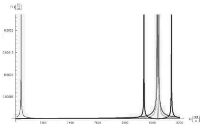
Fig. 8. Dynamical flexibility of the fixed rod vibrating longitudinally in transportation
