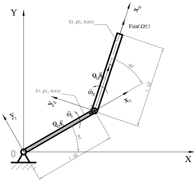
Fig. 3. The two-linked manipulator loaded by a longitudinal force in transportation
