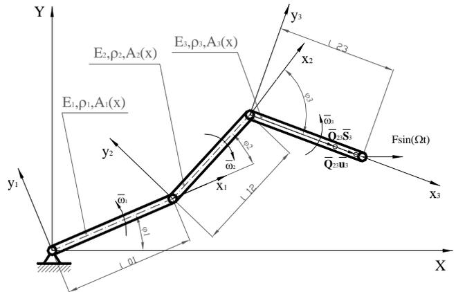
Fig. 4. The three-linked manipulator loaded by a longitudinal force in transportation
