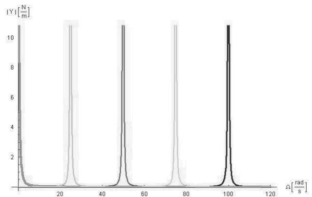
Fig. 7. Dynamical flexibility of the free rod vibrating longitudinally in transportation
