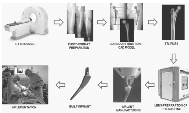
Fig. 2. Manufacturing process using LENS technology principle in medicine
