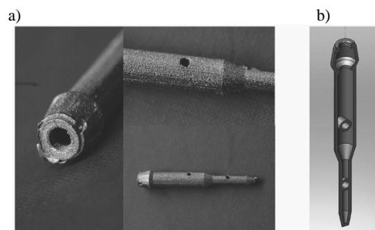
Fig. 6. a) Hollow and thin walled (1 mm) LENS prototype, b) CAD model of LENS prototype
