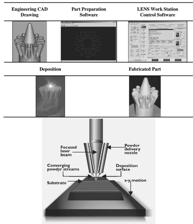
Fig. 1. Process steps and schematic diagram of the LENS technology
