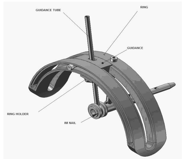
Fig. 5. Nail with groove head and attendance instruments
