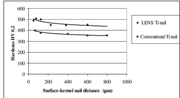
Fig. 8. Hardness of LENS and conventional IM Ti nail trough cross section
