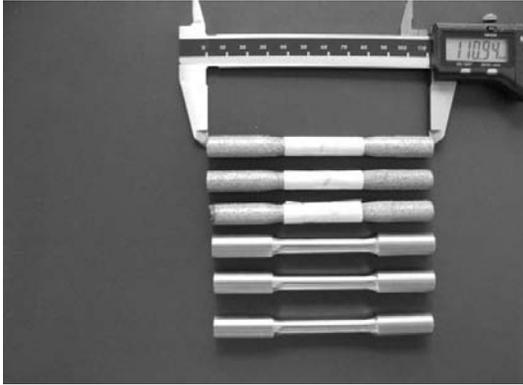
Fig. 7. Testing probes made of wrought titanium and with LENS technology
