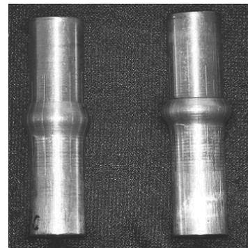
Fig. 6. Formed specimens (punch stroke 4.1mm)
