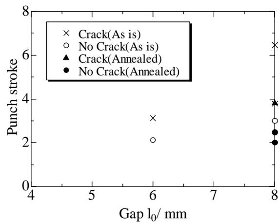
Fig. 12. Forming limit (weld type pipe)
