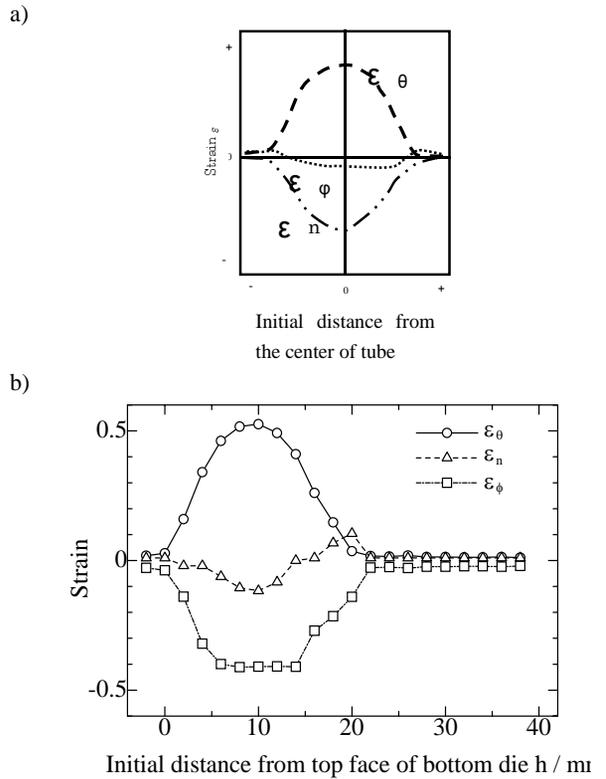
Fig. 2 Typical distributions of the strain [2]: a) hydro-forming, b) proposed process
