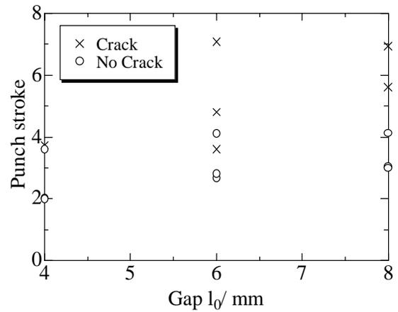
Fig. 11. Forming limit (wire-cut type pipe)
