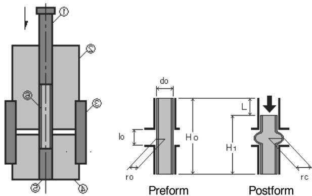
Fig. 5. Dies and specimen: 1-Punch, 2-Upper die, 3-Spacer, 4-Lower die, 5-Knock-out punch
