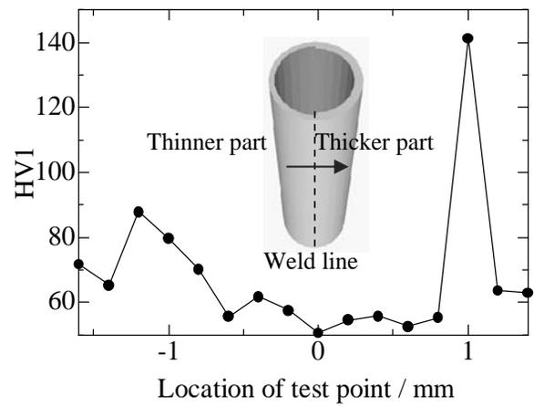
Fig. 10. Hardness distribution on the weld line
