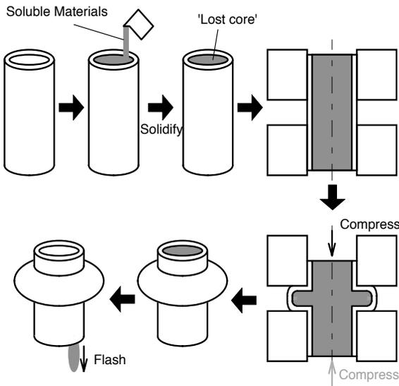
Fig. 1 Lateral extrusion with a lost core [1-2]
