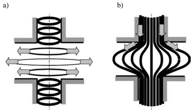
Fig. 3. Typical deformation mechanism [2]: a) hydro-forming without axial compression, b) LELC
