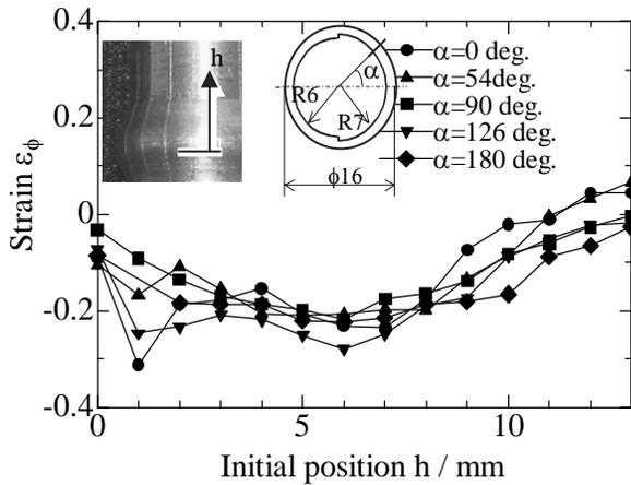
Fig. 8. Meridian strain (Gap 8mm, Punch stroke 4.1mm)
