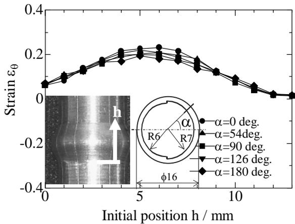
Fig. 7. Circumference strain (Gap 8mm, Punch stroke 4.1mm)
