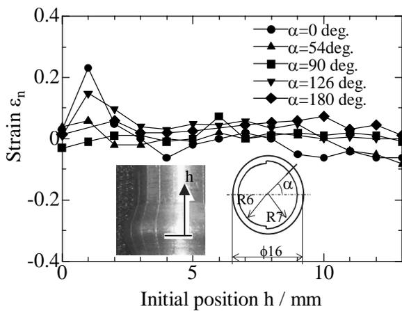
Fig. 9. Reduction of thickness (Gap 8mm, Punch stroke 4.1mm)
