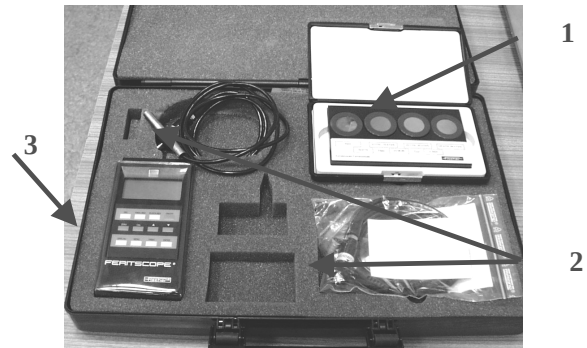
Fig. 36. Complete equipment for measuring the ferrite content, 1 - calibration standards, 2 – connecting cable, 3 - ferritescope [4]
