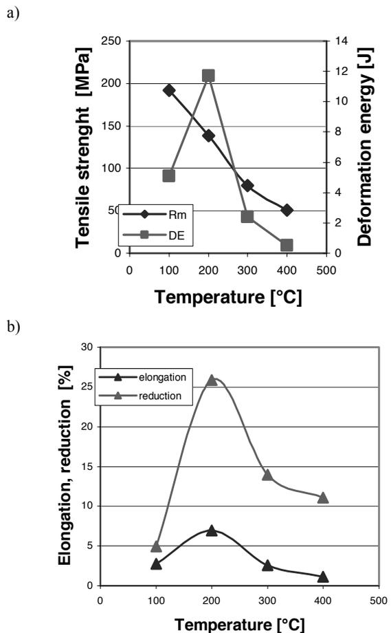
Fig. 2. Temperature dependence of mechanical properties alloy AZ91 after heat treatment: a), b)
