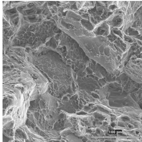
Fig. 16. Analysis of fracture areas of samples A1 at 100°C with use of SEM (the same samples as in the Fig. 9)
