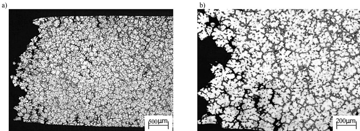
Fig. 7. Microstructure of samples A after tensile test at 300°C: a), b)
