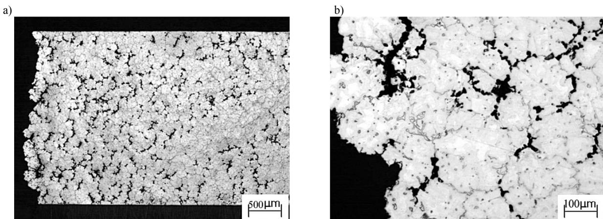
Fig. 8. Microstructure of samples A after tensile test at 460°C: a), b)
