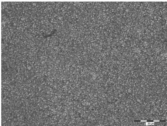
Fig. 20. Microstructure of samples A1 after ECAP method application
