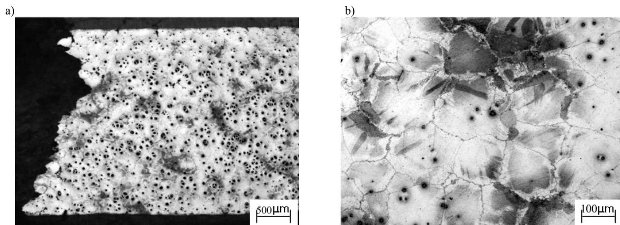
Fig. 10. Microstructure of samples A1 after tensile test at 200°C
