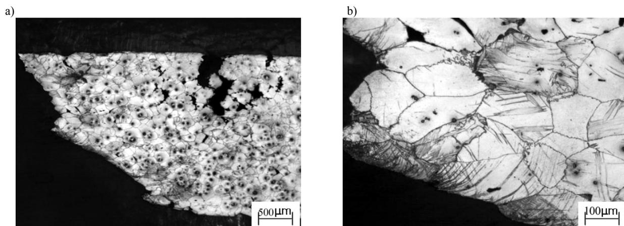
Fig. 9. Microstructure of samples A1 after tensile test at 100°C: a), b)
