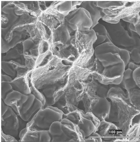
Fig. 18. Analysis of fracture areas of samples A1 at 400°C with use of SEM (the same samples as in the Fig. 11)
