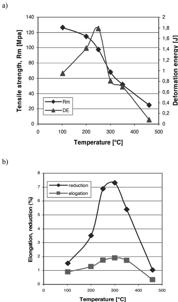
Fig. 1. Temperature dependence of mechanical properties alloy AZ91 as cast state: a), b)
