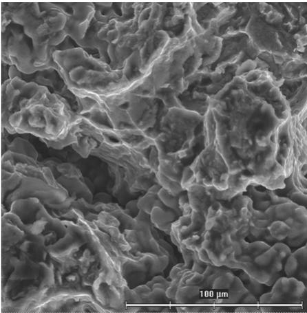
Fig. 13. Analysis of fracture areas of samples A at 250°C with use of SEM (the same samples as in the Fig. 6)
