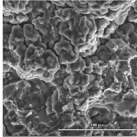
Fig. 15. Analysis of fracture areas of samples A at 100°C with use of SEM (the same samples as in the Fig. 8)
