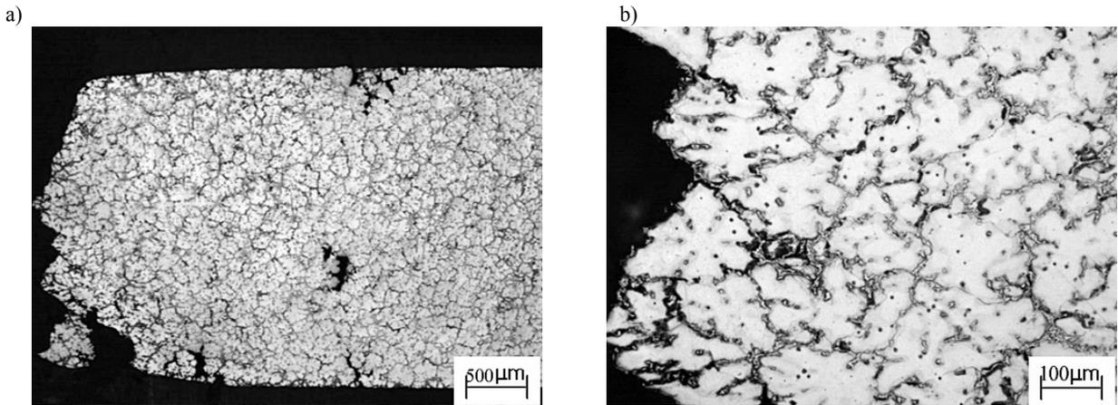
Fig. 6. Microstructure of samples A after tensile test at 250°C: a), b)
