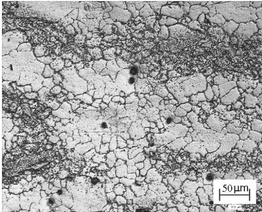
Fig. 19. Microstructure of samples A1 after rolling
