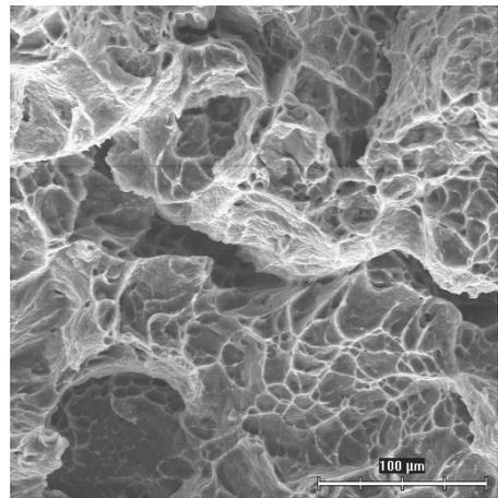
Fig. 17. Analysis of fracture areas of samples A1 at 200°C with use of SEM (the same samples as in the Fig. 10)
