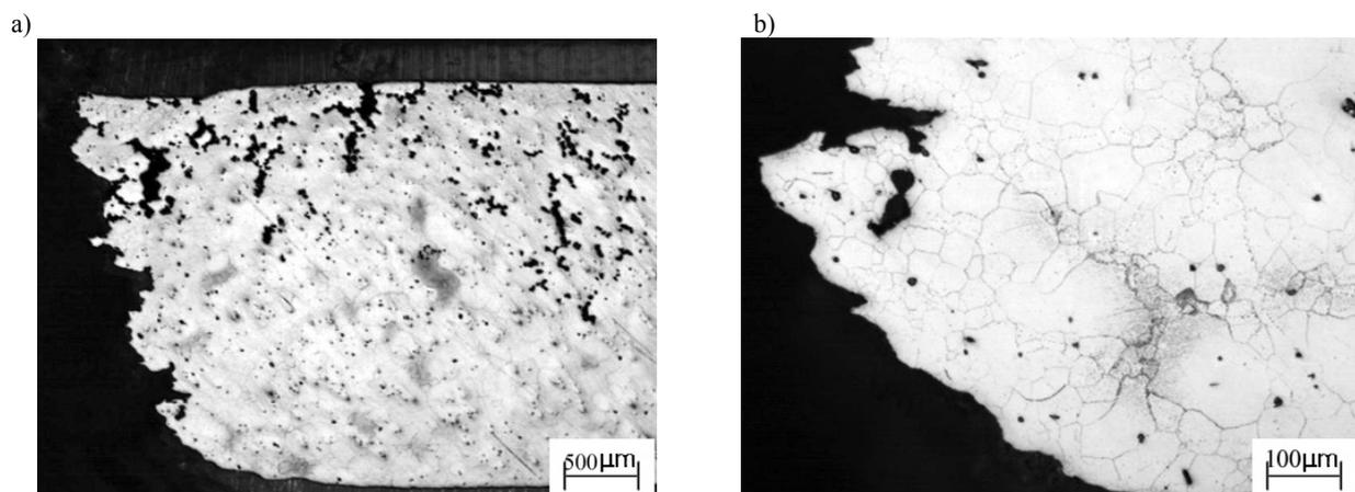
Fig. 11. Microstructure of samples A1 after tensile test at 400°C: a), b)
