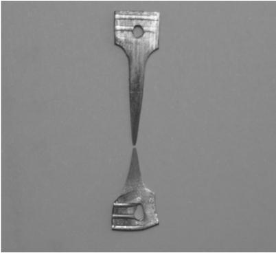
Fig. 3. Shape of ECAP sample after tensile test
