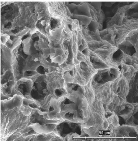
Fig. 14. Analysis of fracture areas of samples A at 300°C with use of SEM (the same samples as in the Fig. 7)
