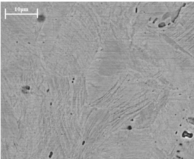
Fig. 14. Elongated  $\gamma$  grains with areas of martensite  $\alpha'$  and some non-metallic inclusions in investigated steel after deformation with a draft of 40%; Etching - Mi17Fe; Mag. 5000x
