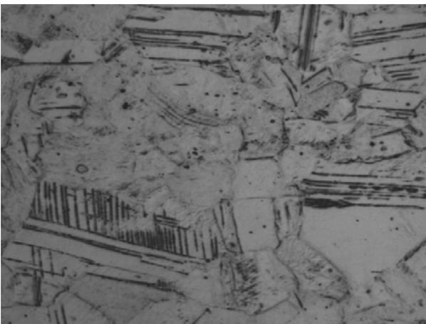
Fig. 2. Structure of the investigated steel after deformation with draft of 20%; Etching - Mi17Fe; Mag. 1000x
