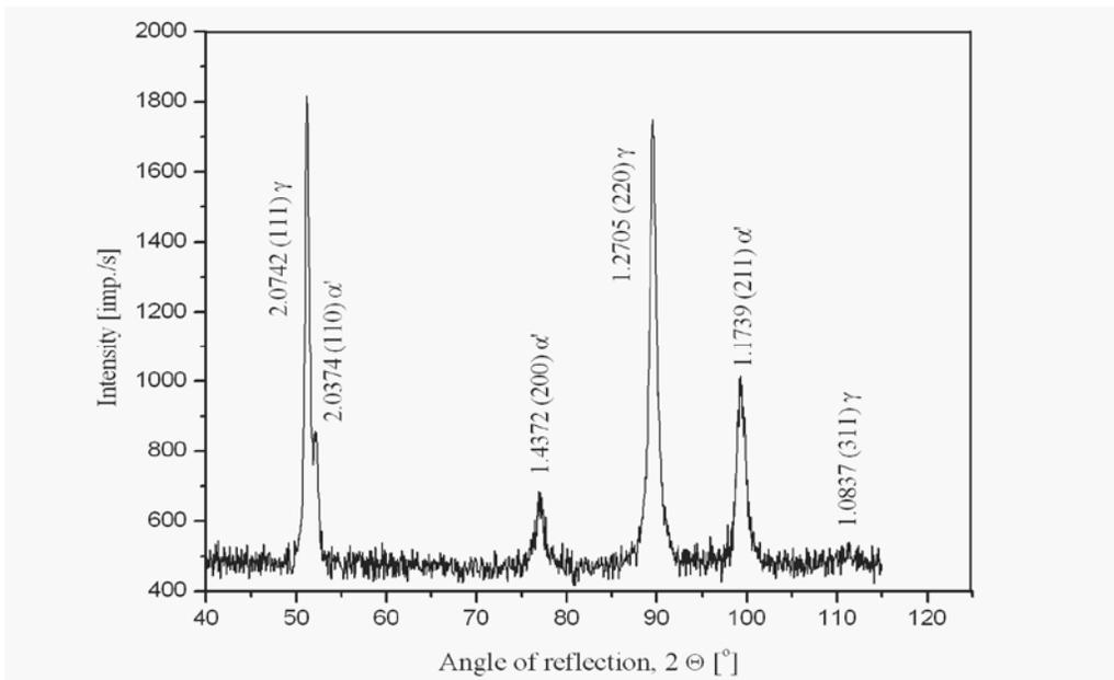
Fig. 7. X-ray diffraction patterns of steel X5CrNi18-9 with a draft of 70%
