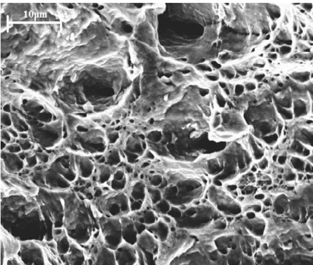
Fig. 10. Transcrystalline ductile fracture of investigated steel type X5CrNi18-9 after deformation with a draft of 20%, Mag. 5000x
