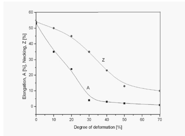
Fig. 6. Changes of the plasticity in the investigated cold rolled steel depending on degree of deformation
