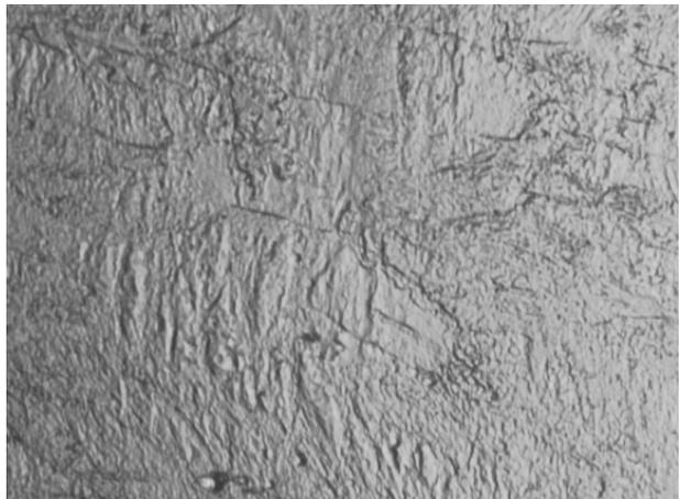
Fig. 4. Structure of the investigated steel after deformation with draft of 70%; Etching - Mi17Fe; Mag. 1000x
