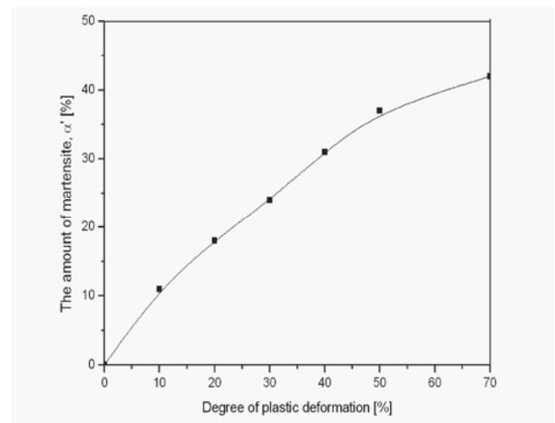
Fig. 8. Dependence of the volume fraction of  $\alpha'$  phase on the degree of plastic deformation of the investigated steel
