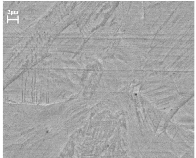
Fig. 15. Areas of parallel plates characteristic for martensite  $\alpha'$  in the investigated steel structure after cold rolling with a draft of 40%; Etching - Mi17Fe; Mag. 8000x
