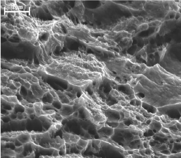
Fig. 13. Ductile fracture of investigated X5CrNi18-9 steel after deformation with a draft of 30%, Mag. 20000x
