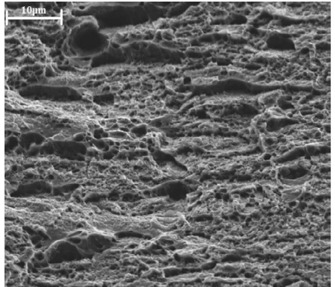
Fig. 11. Mixed fracture of investigated steel type X5CrNi18-9 after deformation with a draft of 30%, Mag. 5000x
