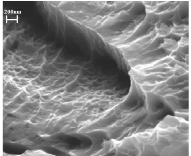
Fig. 12. Terraces on the ductile fracture of investigated steel type X5CrNi18-9 after deformation with a draft of 30%, Mag. 75000x
