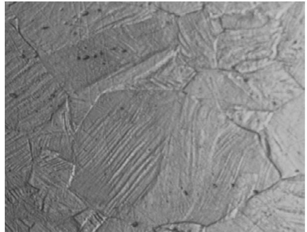
Fig. 3. Structure of the investigated steel after deformation with draft of 30%; Etching - Mi17Fe; Mag. 1000x
