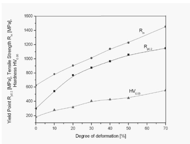
Fig. 5. Changes of the mechanical properties in the investigated cold rolled steel depending on degree of deformation
