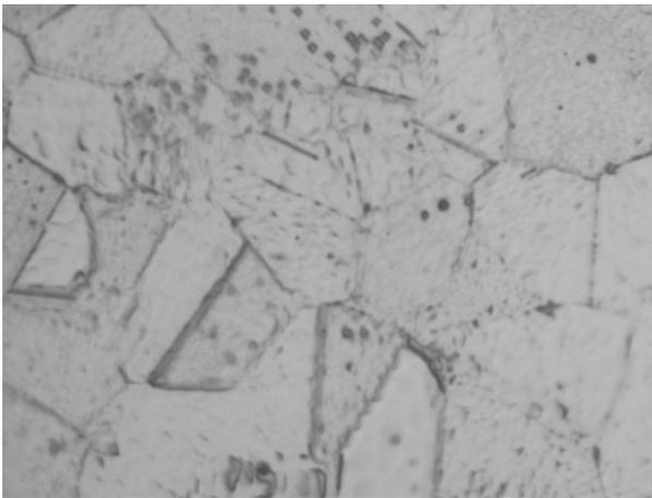
Fig. 1. Supersaturated austenite structure of X5CrNi18-9 steel in the delivered state; Etching - Mi17Fe; Mag. 1000x
