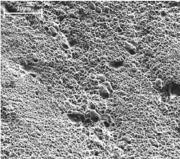
Fig. 9. Ductile fracture of X5CrNi18-9 steel in the delivery state, Mag. 1000x
