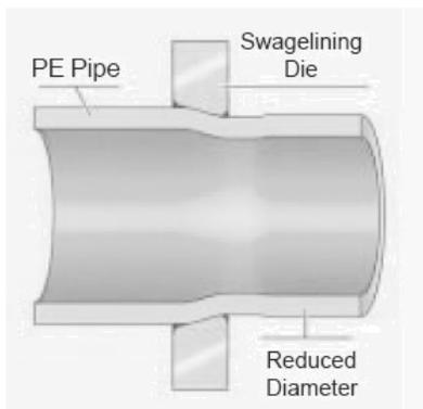
Fig. 4. Action of swageling [15]
