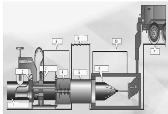
Fig. 3. Idea of renovation in swagelining method [15]: 1 – new PE pipe, 2 – reducing die, 3 – hydraulic pusher, 4 – clamp, 5 – original pipe, 6 – towing cone, 7 – winch, 8 – entry pit, 9 – ground level, 10 – exit pit
