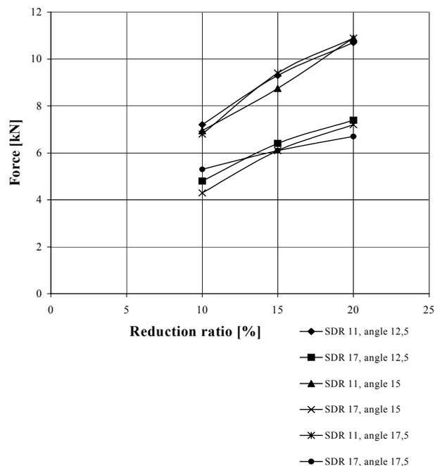
Fig. 7. Drawing force and the reduction ratio
