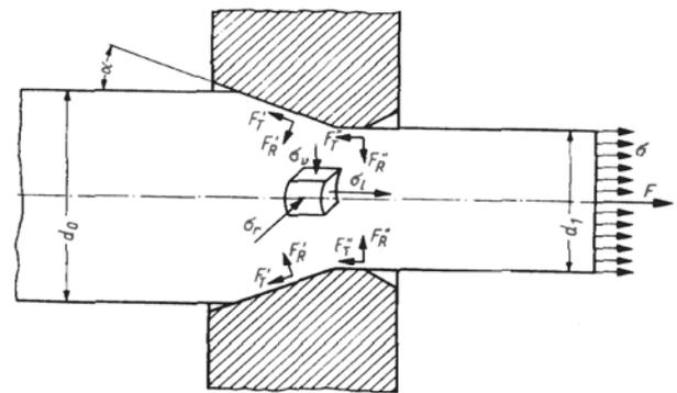
Fig. 5. Forces and stresses in the drawing (sinking) process [25]
