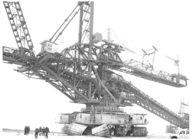
Fig. 3. Breakdown of dumping conveyor's steerable carriage
