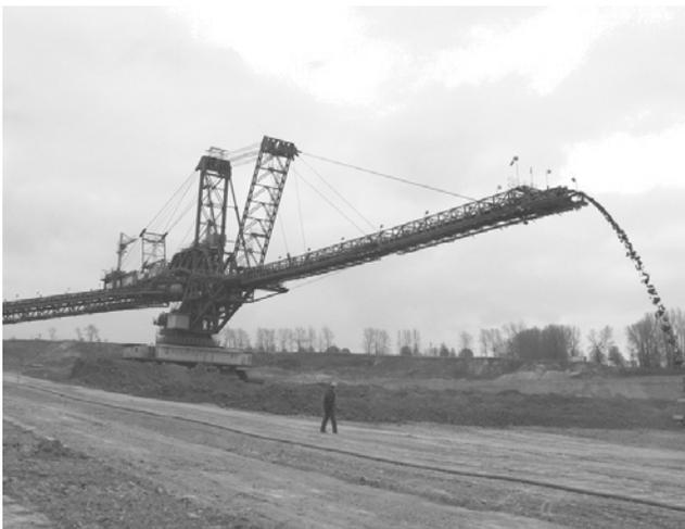
Fig. 2. Dumping conveyor operating in opencast lignite mine
