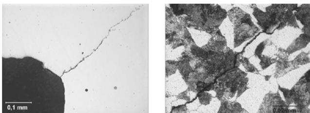
Fig. 22. Edge of lock groove. Light microscopy: a) visible crack initiated in area where cross section changes – unetched condition, b) magnified fragment of area in etched condition, visible crack running along boundaries of ferrite and pearlite grains
