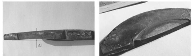
Fig. 11. Deformed elements (plates) protecting against halfshaft slip out
