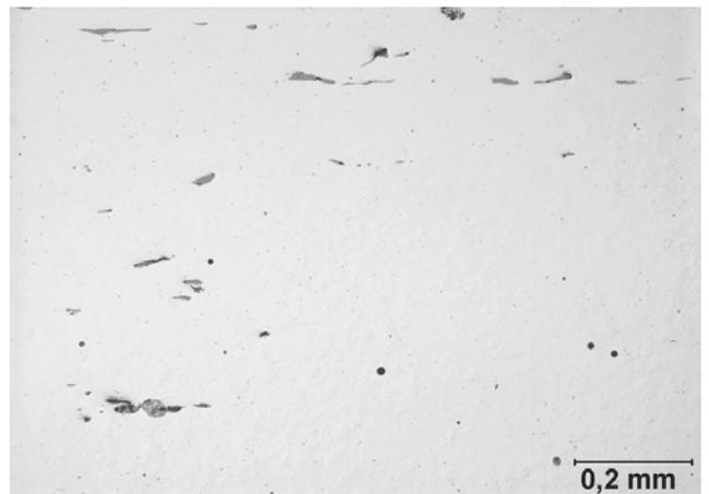
Fig. 19. Non-metallic inclusions uniformly distributed over whole surface of micro-section along direction of plastic working. Unetched condition. Light microscopy
