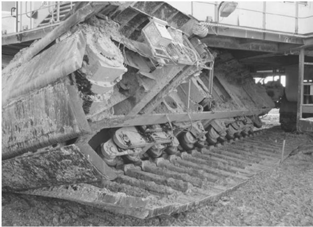
Fig. 6. Breakdown of one carriage: results of steerable carriage breakdown
