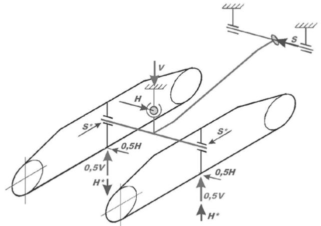
Fig. 8. Forces acting on caterpillar unit during turn
