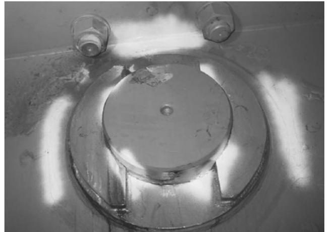
Fig. 10. Halfshaft end - protection against slip out
