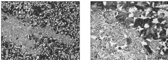
Fig. 21. Etched condition. Light microscopy: a) inhomogeneous pearlitic-ferritic microstructure with features of Widmanstätten structure, b) magnified fragment
