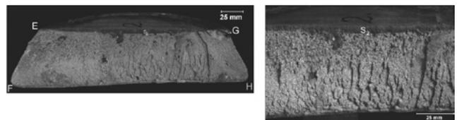
Fig. 15. General view of surface of fracture with marked edges. Symbol S2 marks widest fracture fatigue zone area
