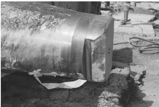
Fig. 7. Damaged halfshaft of steerable carriage
