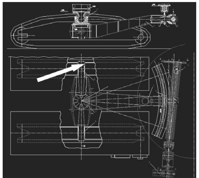
Fig. 4. Schematic of steerable caterpillar unit
