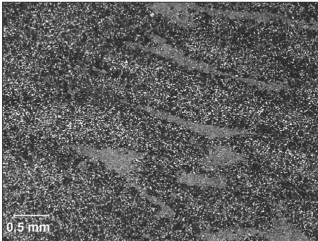
Fig. 20. Inhomogeneous pearlitic-ferritic structure. Etched condition. Light micro-copy
