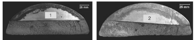
Fig. 13. Fragments broken off caterpillar halfshaft – element 1 and 2
