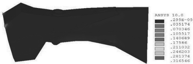
Fig. 12. Strain distribution in bone - compression screws system x100% - Ti-6Al-4V alloy, load step 1
