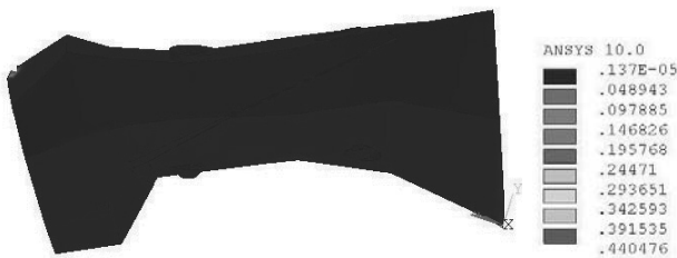
Fig. 14. Strain distribution in bone - compression screw systems x100% - Ti-6Al-4V alloy, load step 2
