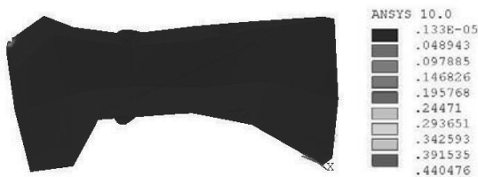
Fig. 21. Strain distribution in bone - compression screws system x100% - Cr-Ni-Mo stainless steel, load step 2
