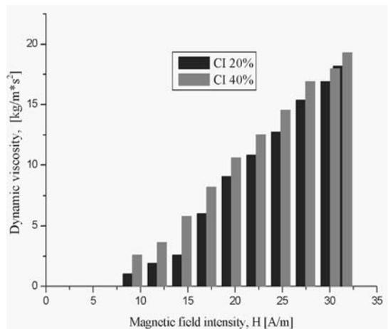
Fig. 9. Dependence of MR fluid (OKS 1050, 50 mPa-s) dynamic viscosity on the magnetic field intensity
