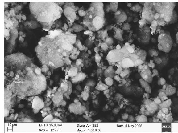
Fig. 5. Silicon dioxide (Aerosil 200)
