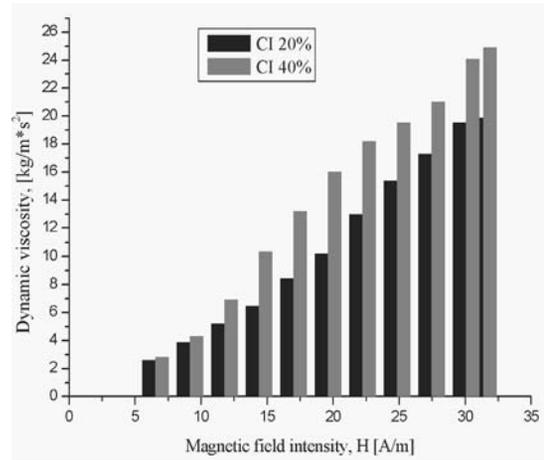
Fig. 10. Dependence of MR fluid (OKS 1050, 500 mPa-s) dynamic viscosity on the magnetic field intensity
