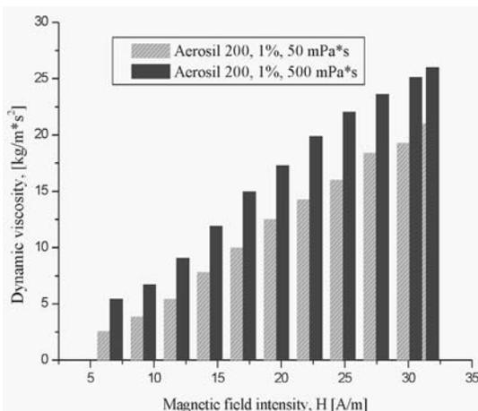
Fig. 14. The influence of carrier liquid viscosity on the dynamic viscosity of MR fluid (CI 40%)
