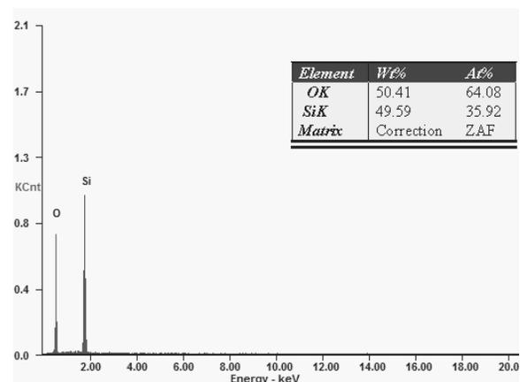
Fig. 6. SEM morphology and special pointwise microanalysis of the chemical composition of fumed silica (Aerosil 200)
