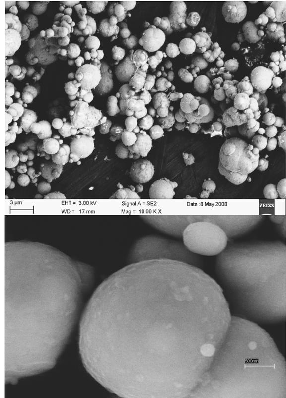
Fig. 3. Scanning electron micrograph of carbonyl iron particles used to prepare MR fluids. Magnification 10 000x and 75 000x
