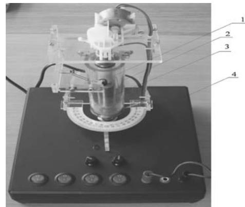
Fig. 2. Apparatus for MR effect measurement. 1 - shaft (drive) and inner cylinder, 2 - outer cylinder, 3 - coil, 4 - needle and angular displacement scale
