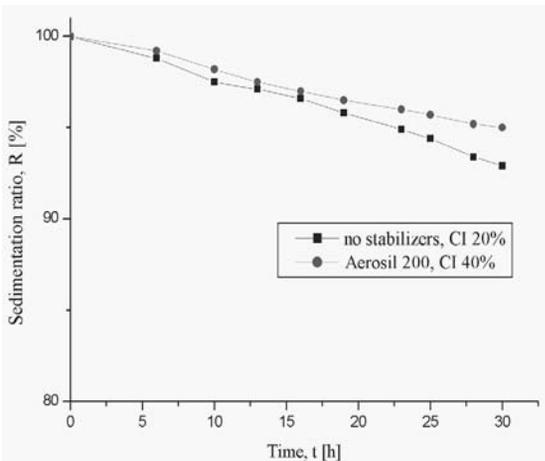
Fig. 8. Sedimentation ratio R of MR fluid (OKS 1050, 500 mPa-s)
