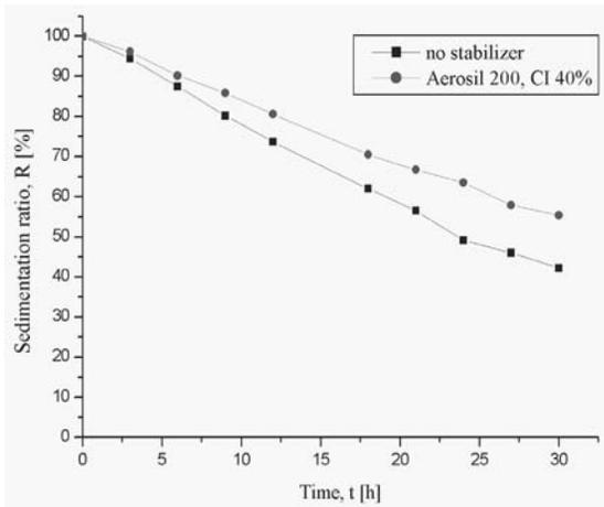
Fig. 7. Sedimentation ratio R of MR fluid (OKS 1050, 50 mPa-s)
