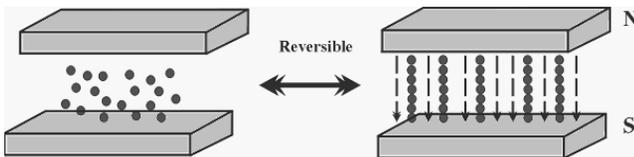
Fig. 1. Micro-structures of MR fluids without/with external magnetic field [8]
