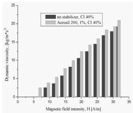
Fig. 11. The influence of the stabilizer on the dynamic viscosity of MR fluid (OKS 1050, 50 mPa-s)
