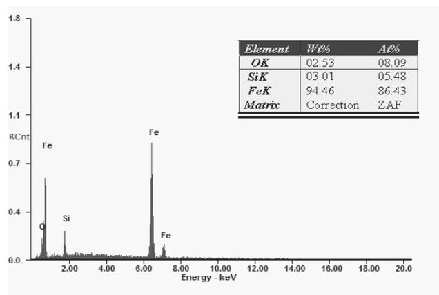
Fig. 4. SEM morphology and special pointwise microanalysis of the chemical composition of the carbonyl iron
