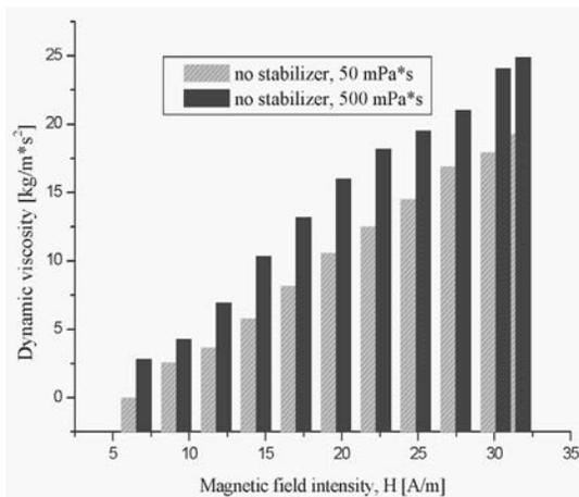
Fig. 13. The influence of carrier liquid viscosity on the dynamic viscosity of MR fluid (CI 40%)
