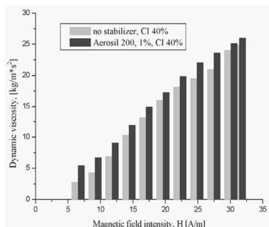
Fig. 12. The influence of the stabilizer on the dynamic viscosity of MR fluid (OKS 1050, 500 mPa-s)
