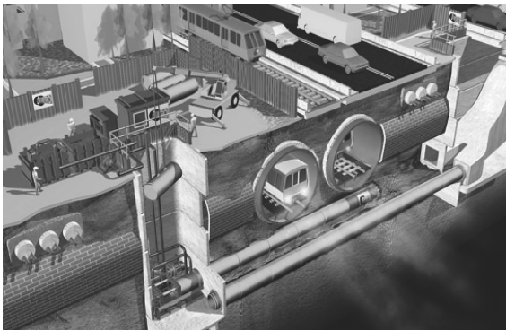
Fig. 1. Microtunneling with fluent excavation material transportation [1]
