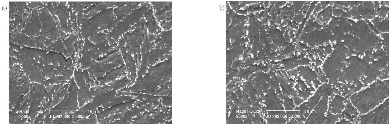
Fig. 13. Microstructure of X10CrWMoVNb9-2 steel after annealing 5000h: a) in temperature 600°C, b) in temperature 650°C observed in scanning electron microscope
