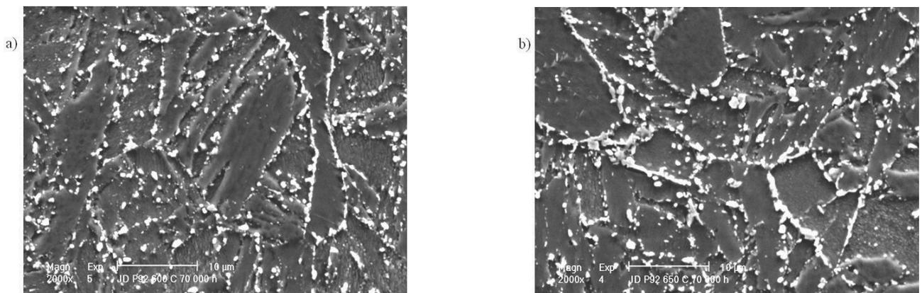
Fig. 15. Microstructure of X10CrWMoVNb9-2 steel after annealing 70000h: a) in temperature 600°C, b) in temperature 650°C observed in scanning electron microscope
