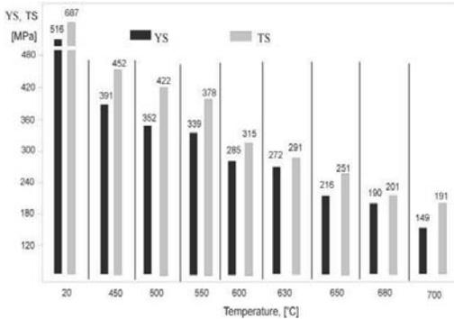
Fig. 1. Tensile strength  $T_s$  and yield point  $Y_s$  versus the examination temperature  $T_b$  of investigated pipe from X10CrWMoVNb9-2 (P92) steel
