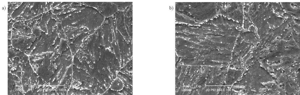
Fig. 11. Microstructure of X10CrWMoVNb9-2 steel after annealing 100h: a) in temperature 600°C, b) in temperature 650°C observed in scanning electron microscope
