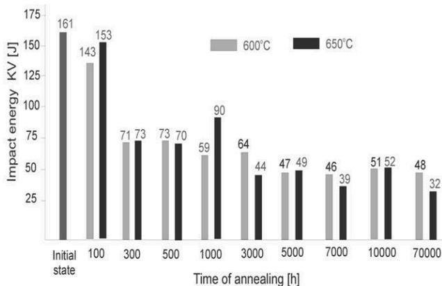
Fig. 5. Influence of annealing time in temperature of 600°C and 650°C on the impact strength for X10CrWMoVNb9-2 steel
