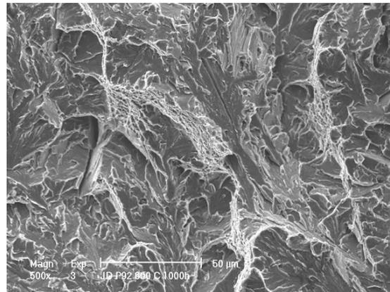
Fig. 7a. Fracture of impact sample of X10CrWMoVNb9-2 steel after 1000h annealing in temperature 600 °C (impact energy 59 J)
