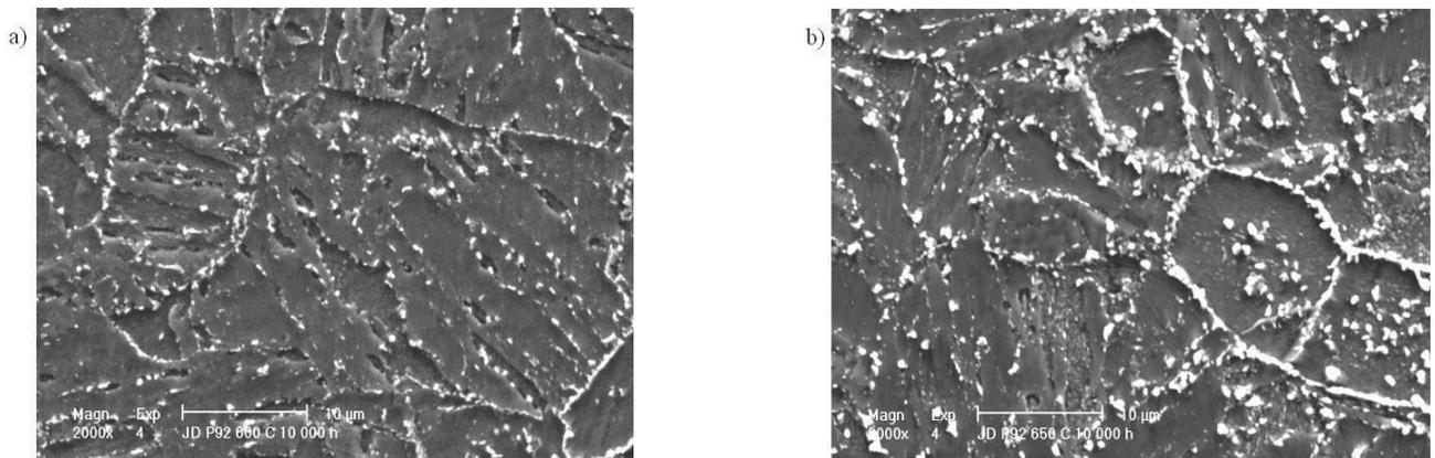
Fig. 14. Microstructure of X10CrWMoVNb9-2 steel after annealing 10000h: a) in temperature 600°C, b) in temperature 650°C observed in scanning electron microscope
