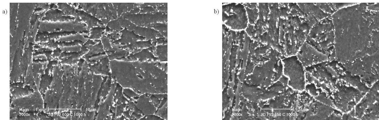
Fig. 12. Microstructure of X10CrWMoVNb9-2 steel after annealing 1000h: a) in temperature 600°C, b) in temperature 650°C observed in scanning electron microscope
