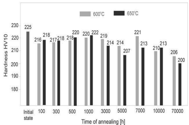
Fig. 10. The influence of annealing time in temperature 600°C and 650°C on X10CrWMoVNb9-2 steel hardness
