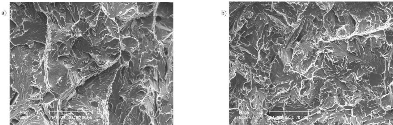
Fig. 9. Fracture of impact sample of X10CrWMoVNb9-2 steel after 70000h annealing: a) in temperature 600°C (impact energy 48 J) b) in temperature 660°C (impact energy 32 J)
