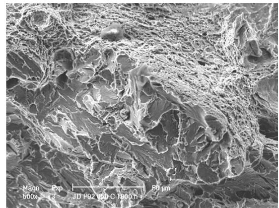
Fig. 7b. Fracture of impact sample of X10CrWMoVNb9-2 steel after 1000h annealing in temperature 650 °C (impact energy 90 J)
