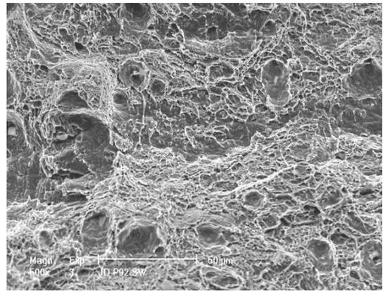
Fig. 6. Fracture of impact sample of X10CrWMoVNb9-2 steel in initial state (impact energy 161 J)
