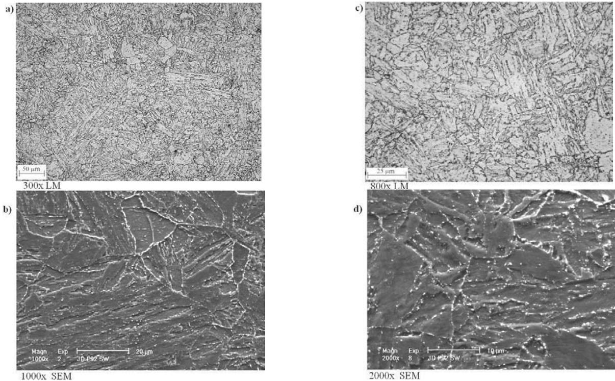
Fig. 3. Microstructure of X10CrWMoVNb9-2 steel in the initial state (N+0) observed: a)light microscope (magn 300x) b) scanning electron microscope (magn 1000 and 2000x)
