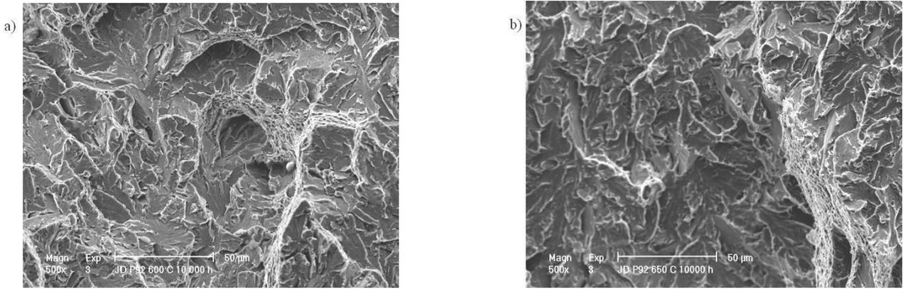
Fig. 8. Fracture of impact sample of X10CrWMoVNb9-2 steel after 10000h annealing : a) in temperature 600°C (impact energy 51J) b) in temperature 660°C (impact energy 52 J)
