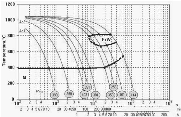
Fig. 4. CCT diagram for X10CrWMoVNb9-2 steel
