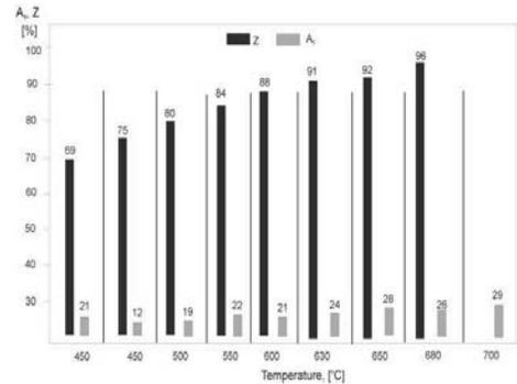
Fig. 2. Results of elongation  $A_5$  and reduction of area  $Z$  during the tensile strength test in the temperature 700°C of investigated pipe from X10CrWMoVNb9-2 (P92)
