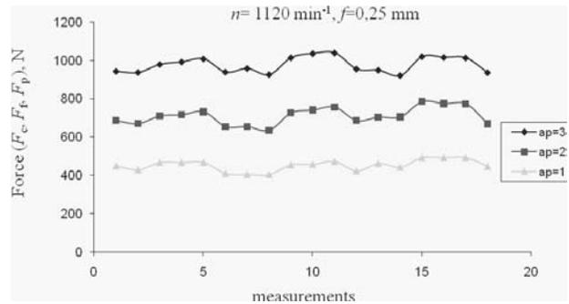
Fig. 11. Force vs. depth of cutting diagram
