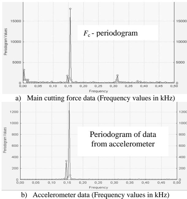
Fig. 6. Signals from accelerometers and force meters after FFT
