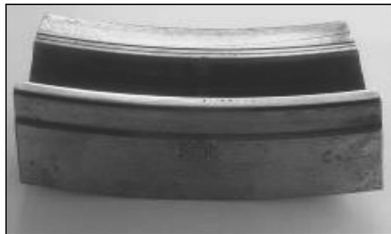
Fig. 2. Outer bearing ring test sample
