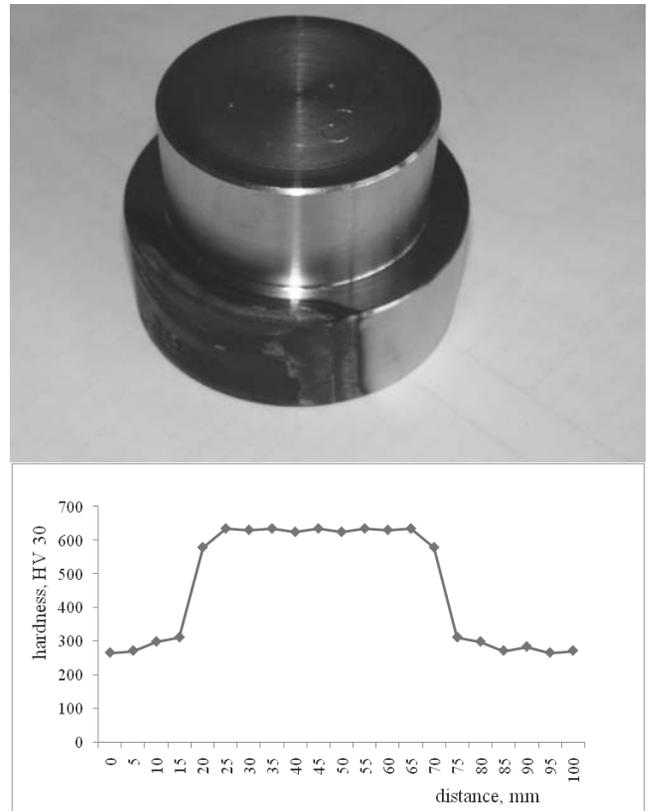
Fig. 5. The test sample after hardening, and the hardness profile
