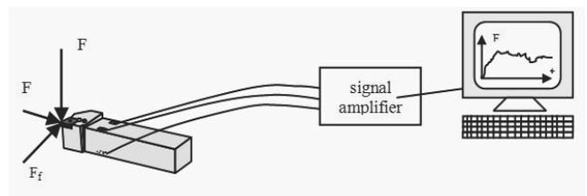
Fig. 8. Force measuring system
