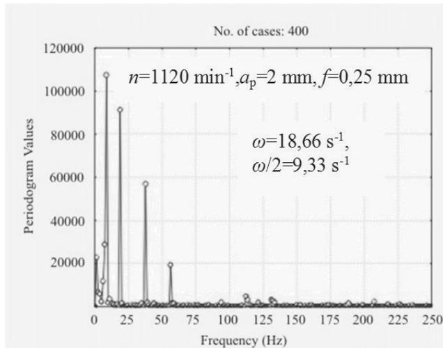
Fig. 10. FFT diagram of force measurement
