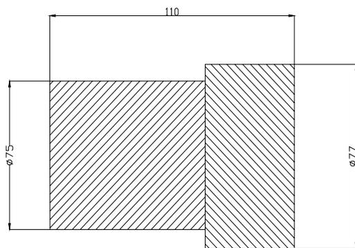
Fig. 4. Geometry of the test sample
