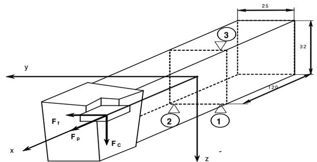
Fig. 7. Strain gages layout
