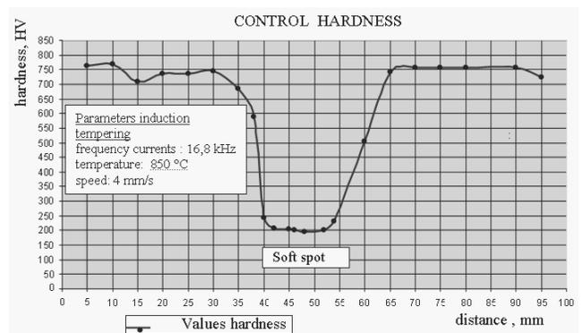
Fig. 3. Hardness profile of outer ring
