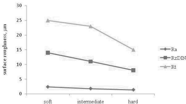
Fig.13. Roughness measuring results
