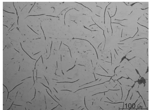
Fig. 13. Microstructure of grey cast iron EN GJL-300 after cast to shell mould (sample II): measurement field 3
