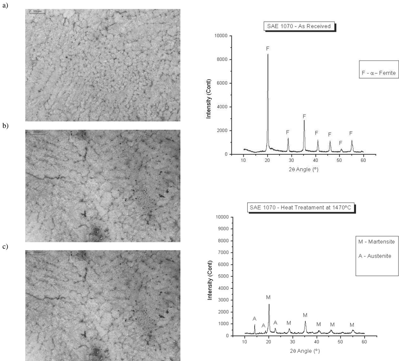
Fig. 4. Microstructures of SAE 1070 steel (optical microscopy) and correspondent XRD patterns, in different conditions: a) as-cast, b) after heat treatment at 1470°C, 0 min, c) after heat treatment at 1470°C, 20 min. Quenched in water
