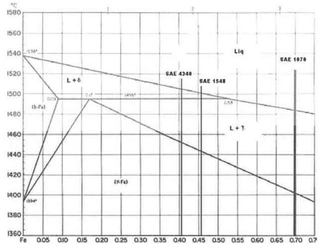
Fig. 2. General phase diagram for Fe-C binary system [12]. Fe-C compositions of investigated steels are indicated
