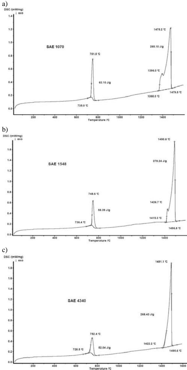
Fig. 1. DSC curves of the studied steels: a) SAE 1070, b) SAE 1548 and c) SAE 4340. Heating rate: 10°C/min
