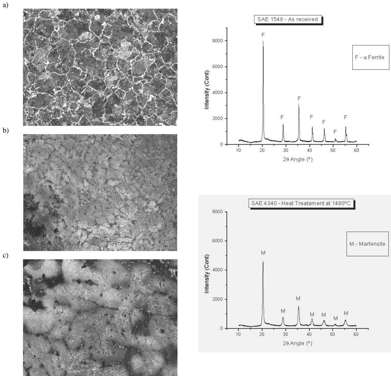
Fig. 5. Microstructures of SAE 1548 steel (optical microscopy) and correspondent XRD patterns, in different conditions: (a) as-cast; (b) after heat treatment at 1480°C, 0 min; (c) after heat treatment at 1480°C, 20 min. In (b) and (c) cases samples were quenched in water
