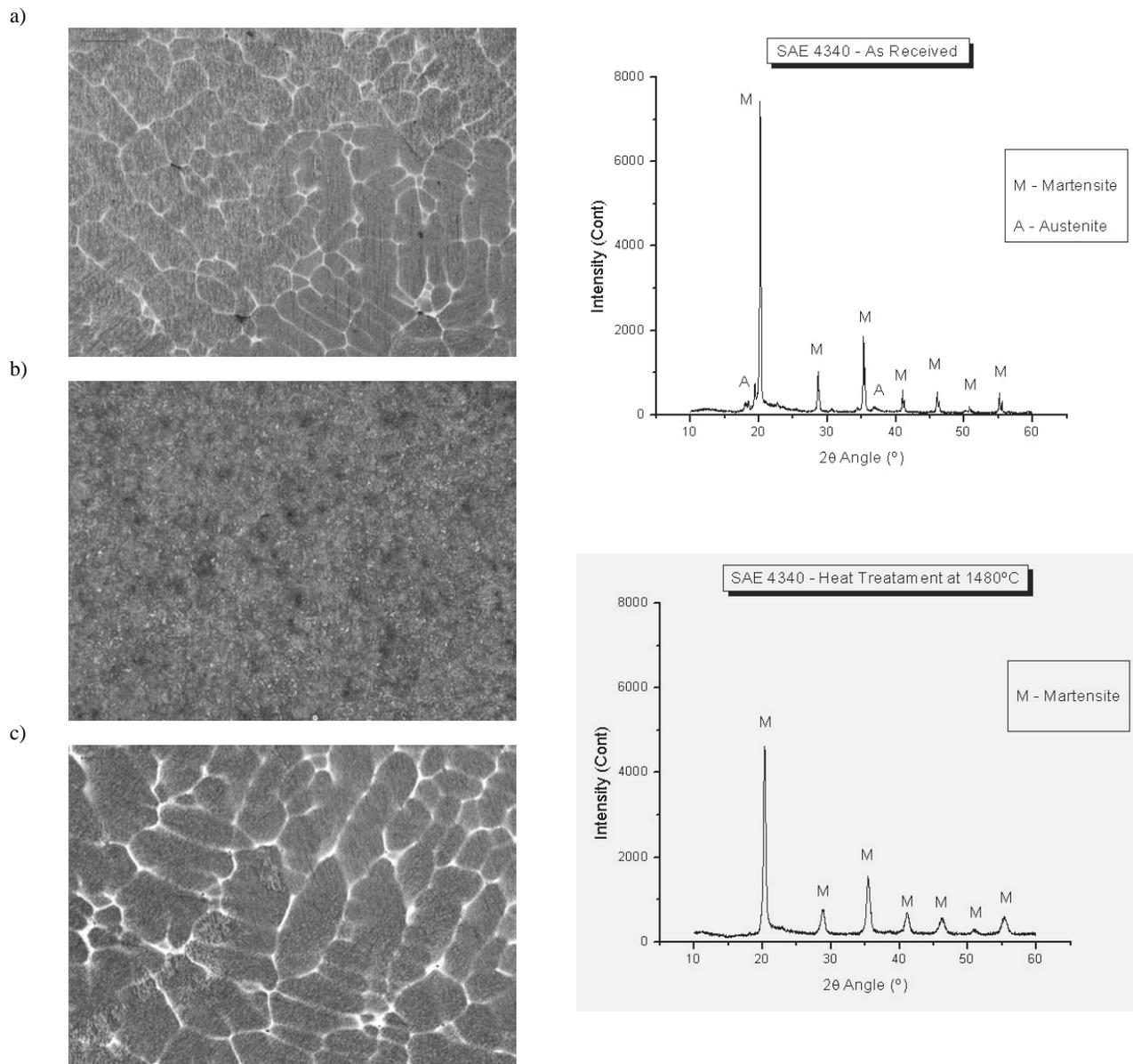
Fig. 6. Microstructures of SAE 4340 steel (optical microscopy) and correspondent XRD pattern, in different conditions: a) forged, b) after heat treatment at 1480°C, 0 min, c) after heat treatment at 1480°C, 20 min. In (b) and (c) cases samples were quenched in water
