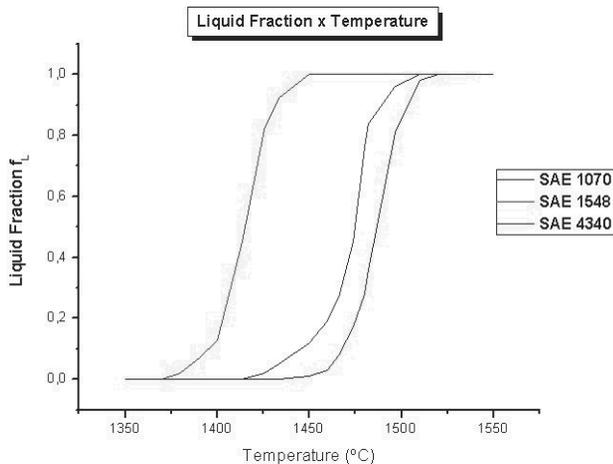
Fig. 3. Variation of liquid fraction with temperature within solidification range of SAE 1070, 1548 and 4340 steels
