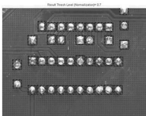
Fig. 12. An example of detected solder joints from database 2
