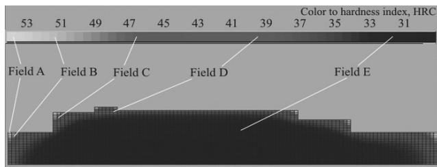
Fig. 4. Distributions of microstructure and mechanical properties fields of the workpiece for quenching in oil;  $H = 0.25$
