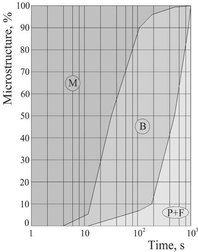
Fig. 3. Microstructure compositions vs. time  $t_{8/5}$ ; (P+F) - Pearlite + Ferrite; B - Bainite; M - Martensite
