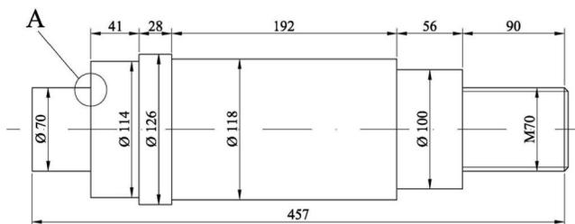
Fig. 1. Workpiece geometry
