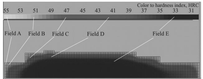
Fig. 5. Distributions of microstructure and mechanical properties fields of the workpiece for quenching in oil;  $H = 0.7$
