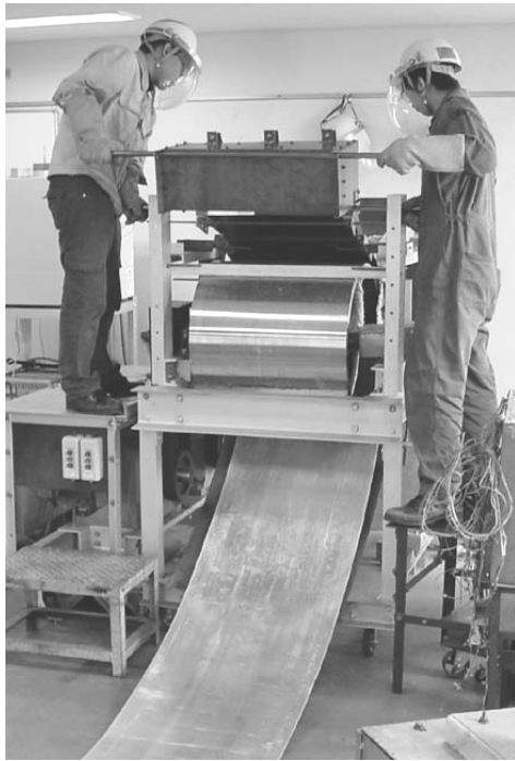
Fig. 13. Roll casting of 600 mm-width 5182 strip at speed of 60 m/min. Roll diameter was 600 mm, and width was 600mm. Structure of the roll is as same as Figure 1c
