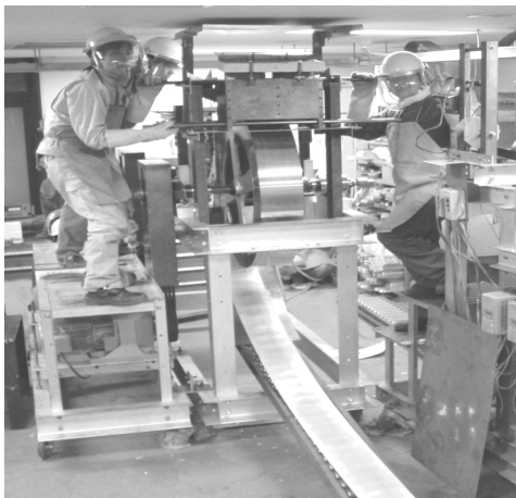
Fig. 2. Photographs of twin roll casters of the present study: a) unequal diameter twin roll caster, b) vertical type high speed twin roll caster in operation of casting. Strip is 5182 and casting speed is 60 m/min
