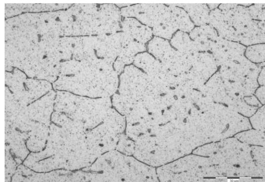
Fig. 12. AlMn1Cu microstructure - initial state
