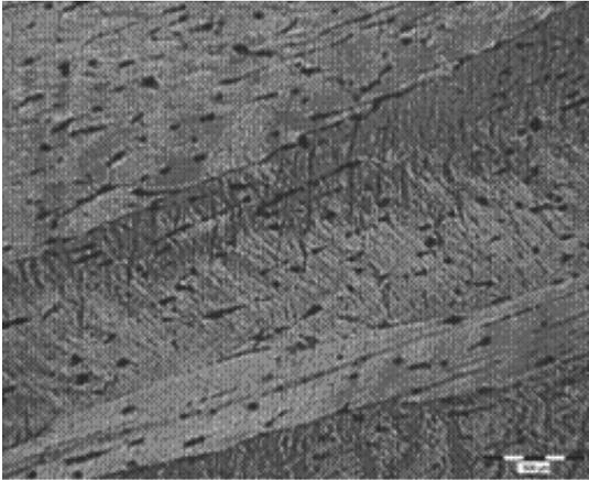
Fig. 13. AlMn1Cu microstructure after the 1<sup>st</sup> pass (deflection 10°)
