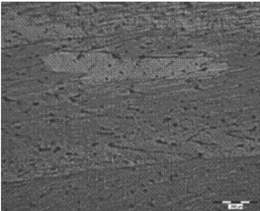
Fig. 14. AlMn1Cu microstructure after the 2<sup>nd</sup> pass (deflection 10°)
