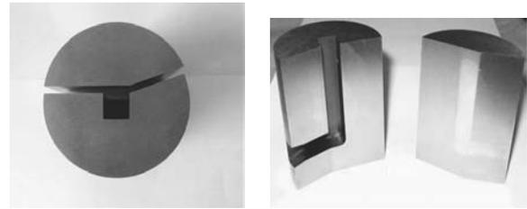
Fig. 1. New geometry of the ECAP dies (axis offset  $20^\circ$ )
