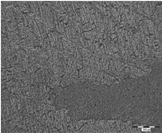
Fig. 20. AlMn1Cu microstructure after the 3<sup>rd</sup> pass, (deflection 10°) - perpendicular
