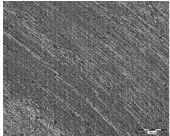
Fig. 22. AlMn1Cu microstructure after the 5<sup>th</sup> pass, (deflection 10°) - perpendicular
