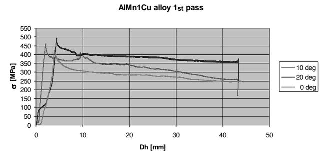
Fig. 7. Influence of the channel deflection on strengthening, first pass
