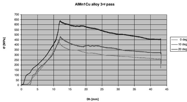
Fig. 9. Influence of the channel deflection on strengthening, third pass
