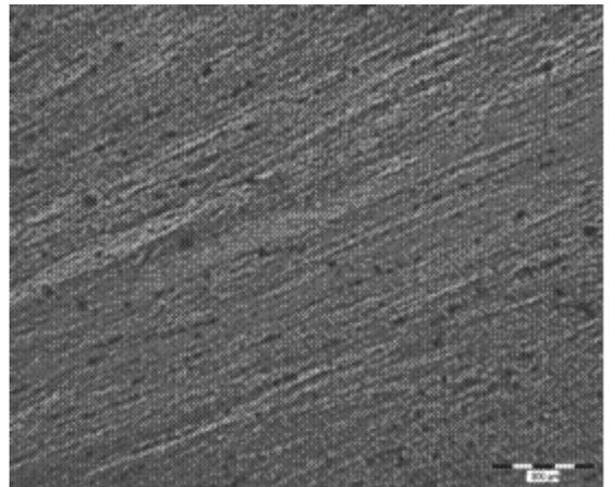
Fig. 17. AlMn1Cu microstructure after the 5th pass (deflection 10°)
