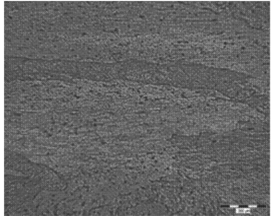
Fig. 16. AlMn1Cu microstructure after the 4<sup>th</sup> pass (deflection 10°)
