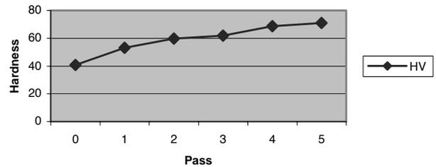
Fig. 25. Hardness of AlMn1Cu after the 5 passes (deflection 20°)
