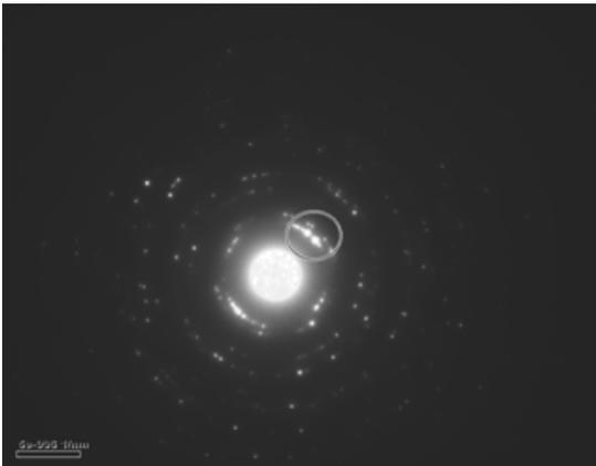
Fig. 24. EM of AlMn1Cu after the 5<sup>th</sup> pass (deflection 10°); a) view of TEM, b) diffraction pattern
