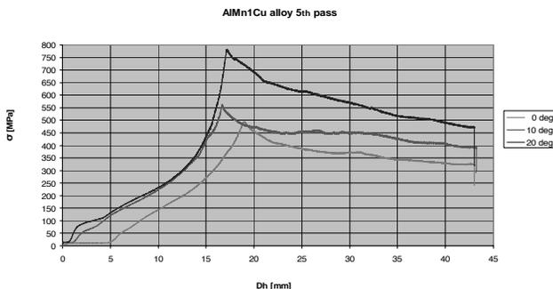
Fig. 11. Influence of the channel deflection on strengthening, fifth pass
