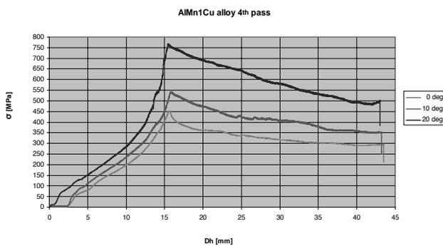
Fig. 10. Influence of the channel deflection on strengthening, fourth pass
