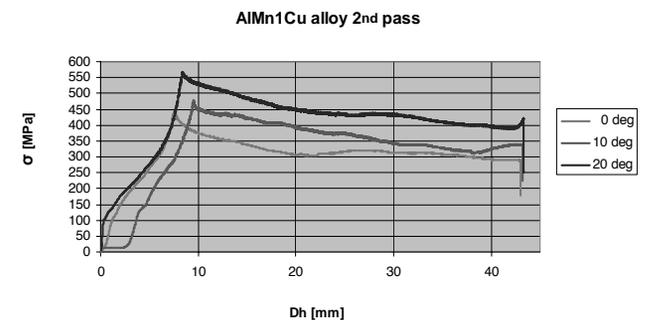
Fig. 8. Influence of the channel deflection on strengthening, second pass
