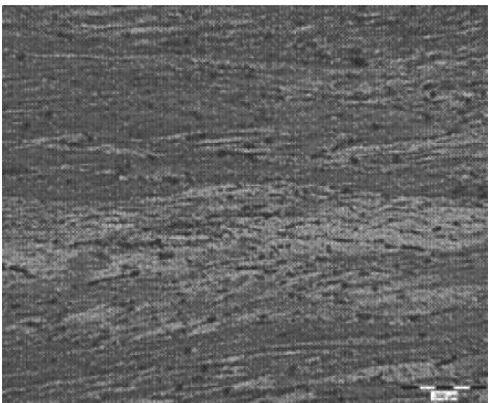
Fig. 15. AlMn1Cu microstructure after the 3<sup>rd</sup> pass, (deflection 10°)
