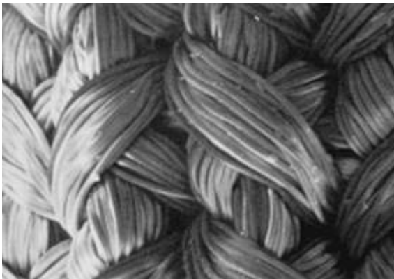
Fig. 4. Close-up photograph ( \times 50 ) of a knitted polyester prosthetic vascular graft [19]
