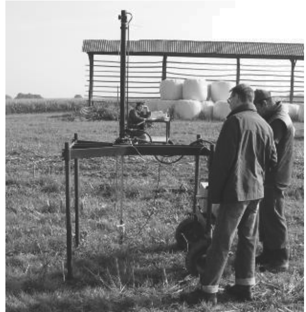
Fig. 2. Measuring of soil resistance with penetrometre
