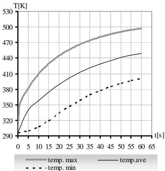
Fig. 8. The diagrams of the maximum, average and minimum values of temperatures of the piston for the  $\lambda = 1.66$  during 60 seconds of the engine work
