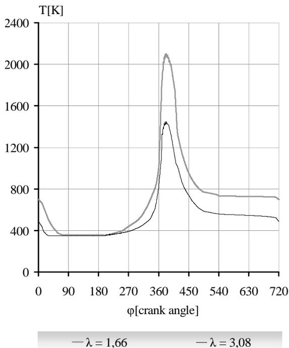
Fig. 2. The diagrams of the average temperature of the working medium for engine speed  $n=2000$  [rpm] and  $\lambda = 1.66$  and  $\lambda = 3.08$
