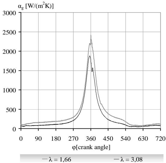
Fig. 1. The diagrams of total surface film conductance in function of crank angle for engine speed  $n = 2000$  [rpm] and  $\lambda = 1.66$  and  $\lambda = 3.08$
