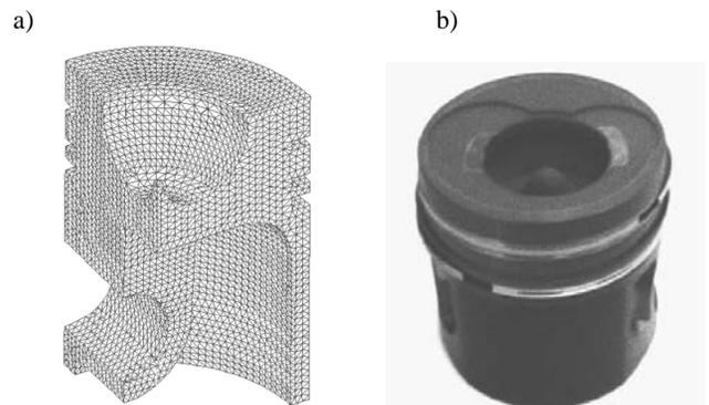
Fig. 4. The piston engine: a) discreet model, b) real element
