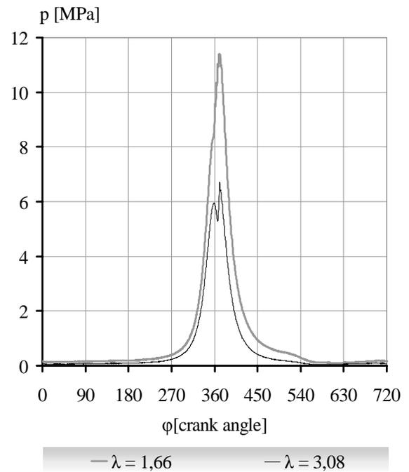
Fig. 3. The diagrams of the indicated pressure for the turbocharged Diesel engine about power rating  $N=85$  [kW] and engine speed  $n=2000$  [rpm] for  $\lambda = 1.66$  and  $\lambda = 3.08$
