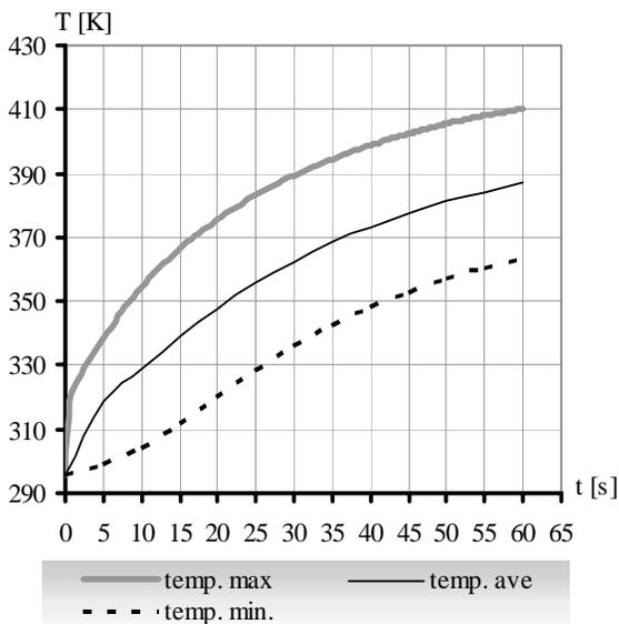
Fig. 9. The diagrams of the maximum, average and minimum values of temperatures of the piston for the  $\lambda = 3.08$  during 60 seconds of the engine work
