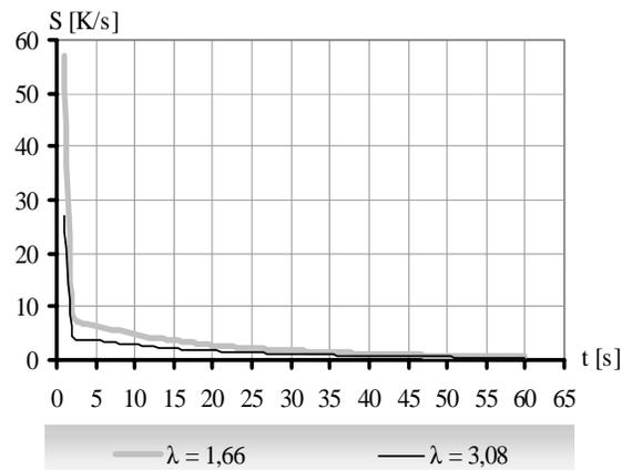
Fig. 10. The speed of the increase temperature of the piston head for two loads of engine during 60 seconds of its work
