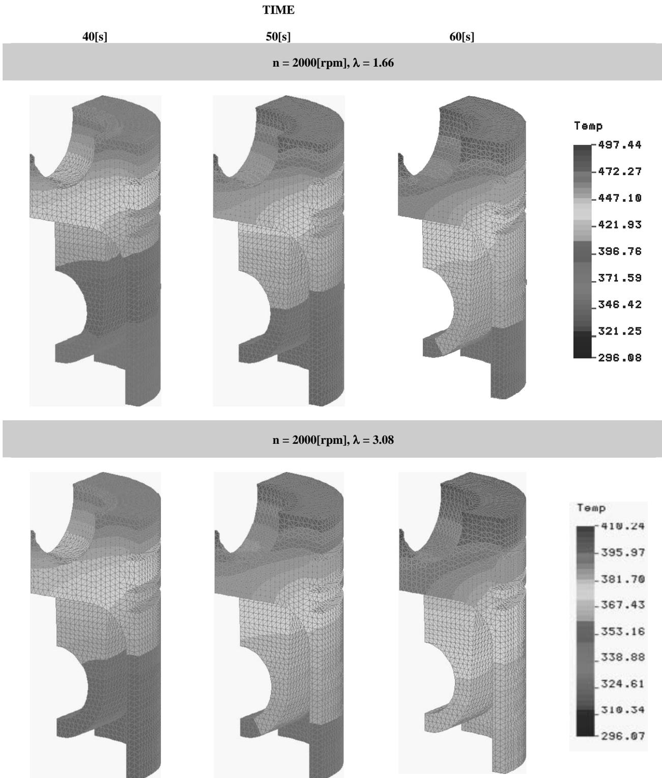
Fig. 7. The following phases warming up of the piston engine
