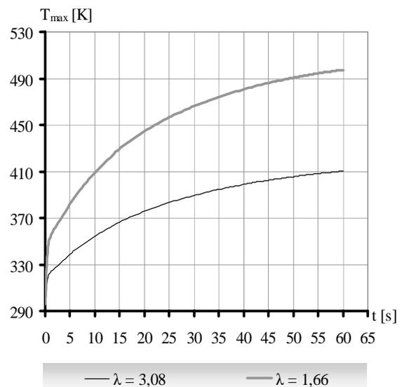
Fig. 11. The comparison of courses of maximum temperature for two loads of engine
