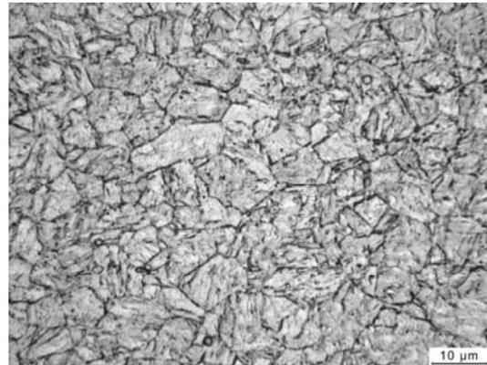
Fig. 1. Microstructure of the cobalt-free maraging steel after hot deformation and heat treatment (annealing and ageing)
