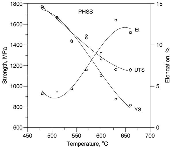
Fig. 9. Tensile properties after cold working and ageing (3 hrs) of the PHSS steel
