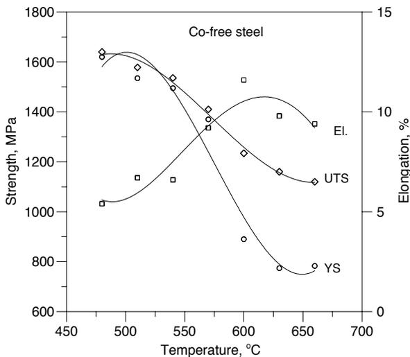
Fig. 10. Tensile properties after cold working and ageing (3 hrs) of the cobalt-free sheet steel
