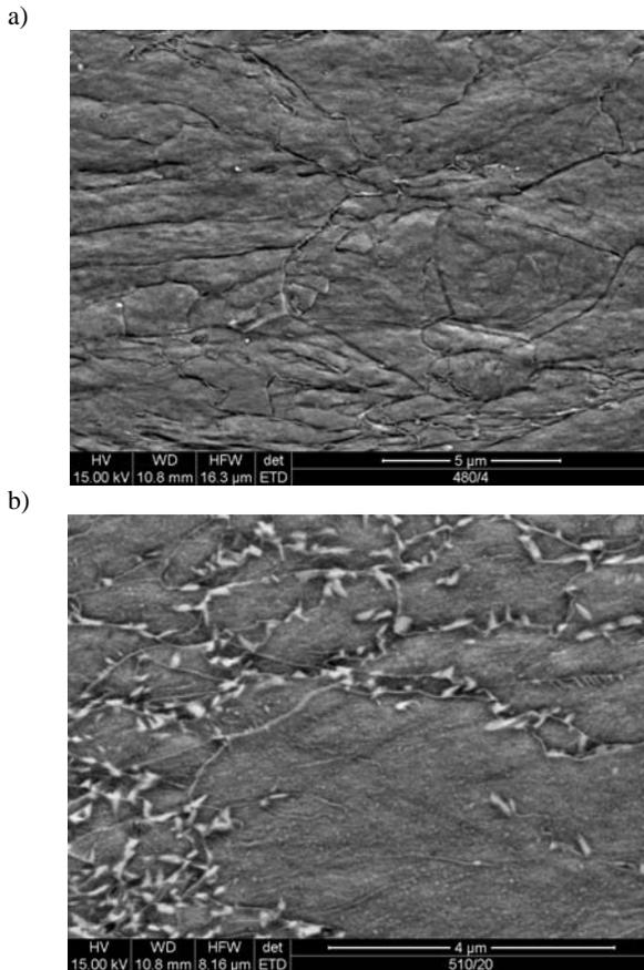
Fig. 7. Scanning electron micrographs of the cobalt-free sheet cold worked 46% and aged at a) 480°C, 3 hrs, ) aged at 510°C, 20 hrs
