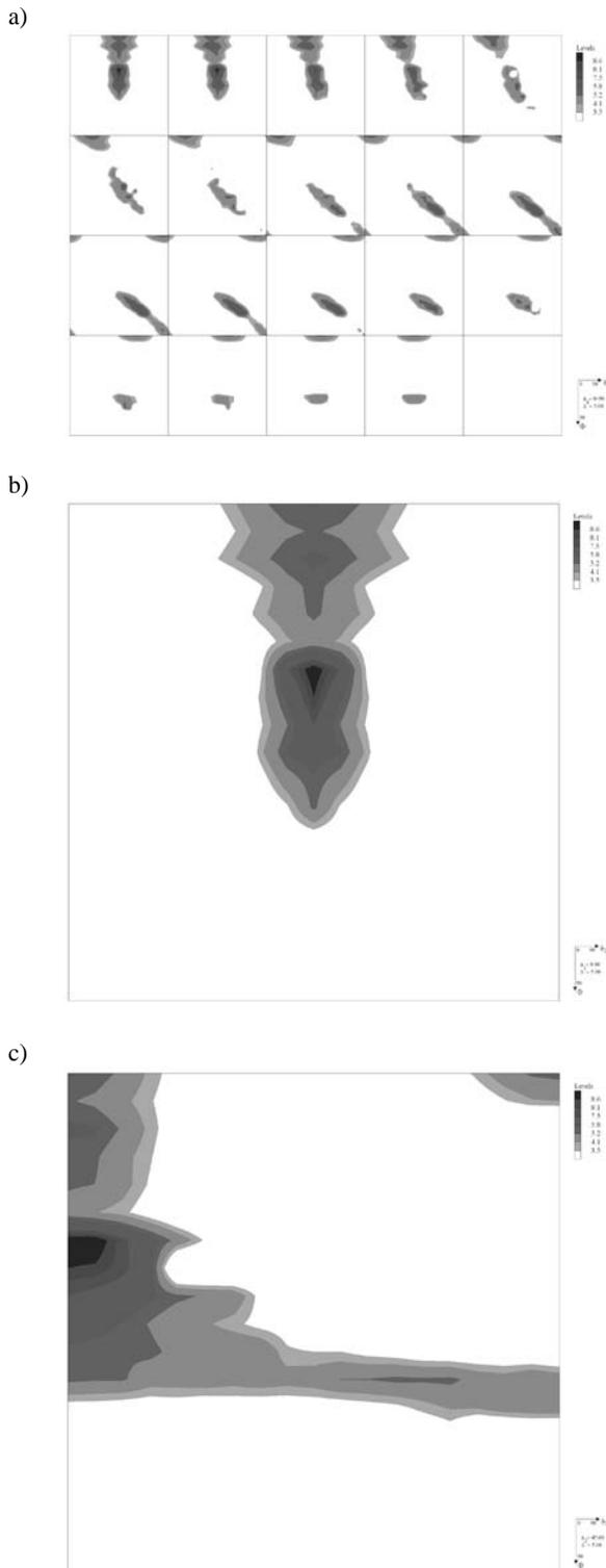
Fig. 4. Orientation distribution function (ODF) representations of the rolling textures of cobalt-free maraging (Fig. 4a – ODF representation for  $\varphi_1 = \text{const}$ , with  $\Delta\varphi_1 = 5^\circ$ , Fig. 4b – ODF section  $\varphi_1 = 0^\circ$ , Fig. 4c – ODF section  $\varphi_2 = 45^\circ$ )
