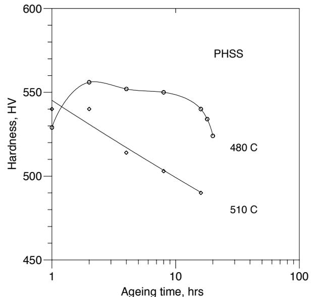
Fig. 5. Hardness (HV30) of the PHSS sheet after cold rolling and ageing at 480°C and 510°C
