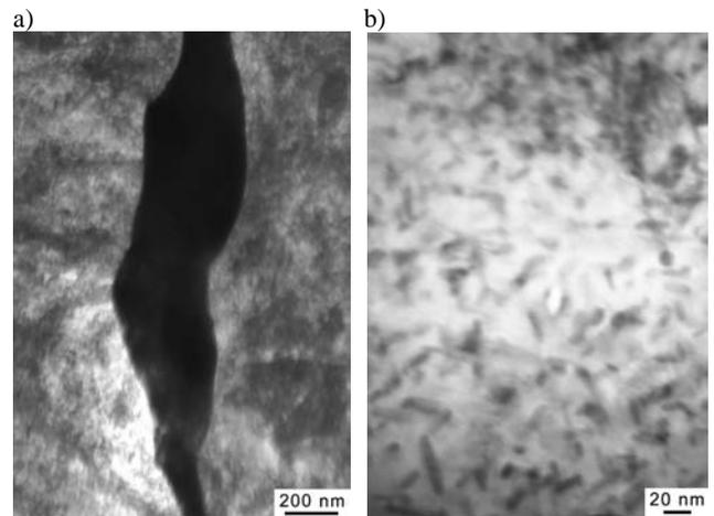
Fig. 8. Transmission electron micrographs of the cobalt-free sheet cold worked 46% and aged at 510°C, 20 hrs. a) reverted austenite in martensite matrix, b) precipitates in martensite matrix
