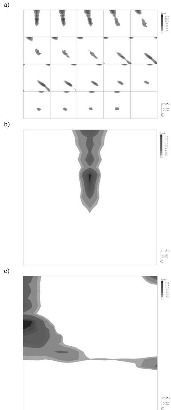
Fig. 3. Orientation distribution function (ODF) representations of the rolling textures of PHSS steel (Fig. 3a – ODF representation for  $\varphi_1 = \text{const}$ , with  $\Delta\varphi_1 = 5^\circ$ , Fig. 3b – ODF section  $\varphi_1 = 0^\circ$ , Fig. 3c – ODF section  $\varphi_2 = 45^\circ$ )
