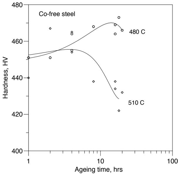
Fig. 6. Hardness (HV30) of the cobalt-free sheet steel after cold rolling and ageing at 480°C and 510°C
