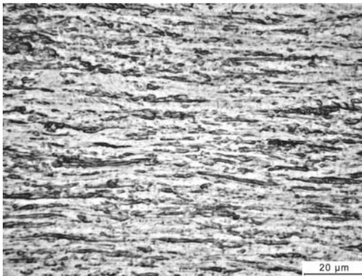
Fig. 2. Microstructure of the PHSS sheet after 74% cold reduction (0.9 mm sheet; polish vertical to sheet surface in the rolling direction)
