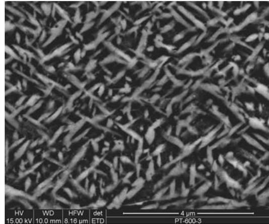
Fig. 11. Scanning electron micrograph of the PHSS sheet aged at 600°C, 3 hrs
