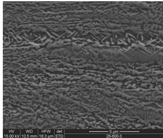
Fig. 12. Scanning electron micrograph of the cobalt-free sheet aged at 600°C, 3 hrs
