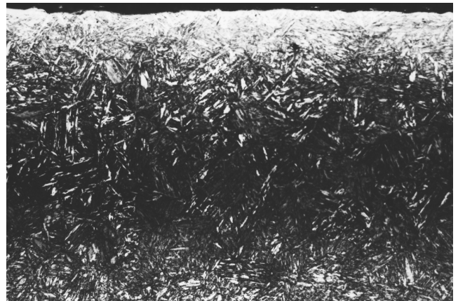
Fig. 7. Microstructure of plasma nitrided layer. Sample 34A2. Compact nitride and diffusion zones. Nital etched
