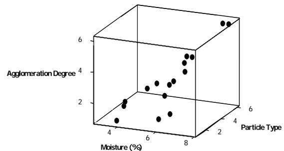
Fig. 5. Scatter plot of agglomeration ( $\hat{y}_3$ ) versus moisture content and particle type
