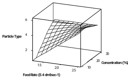
Fig. 4. Response surface plot for the particle type ( $\hat{y}_2$ ) versus sericin concentration and feed rate
