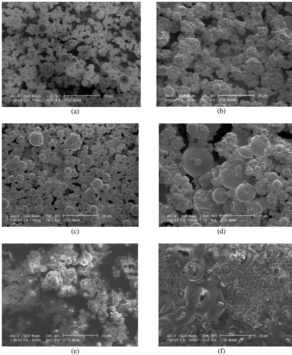
Fig. 1. SEM micrographs for the spray-dried particles with different morphologies: (a) Type 1, (b) Type 2, (c) Type 3, (d) Type 4, (e) Type 5 and (f) Type 6
