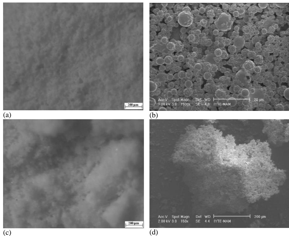
Fig. 2. Representative stereo-microscope images of each category presenting the agglomeration degree; (a) no-agglomeration with agglomeration degree of '1', (b) SEM image of non-agglomerated sample with x1500 magnification and (c) drastic agglomeration with agglomeration degree of '6 (d) the SEM image of a granule from the representative sample with x150 magnification
