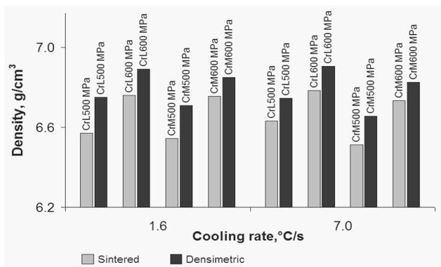
Fig. 7. Comparison between sintered density and density measured with Archimedes' principle of studied compositions (rectangular samples); mean values
