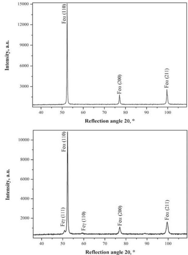
Fig. 8. X-ray diffraction pattern of: a) CrL 500 MPa, medium cooling; b) CrM 500 MPa, high cooling
