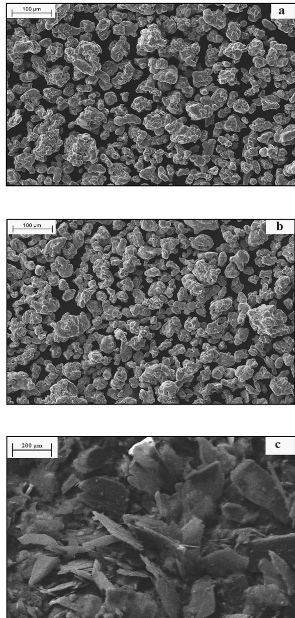
Fig. 3. Micrographs of base powders: a) Astaloy CrL pre-alloyed powder, b) Astaloy CrM pre-alloyed powder, c) GR12 graphite powder
