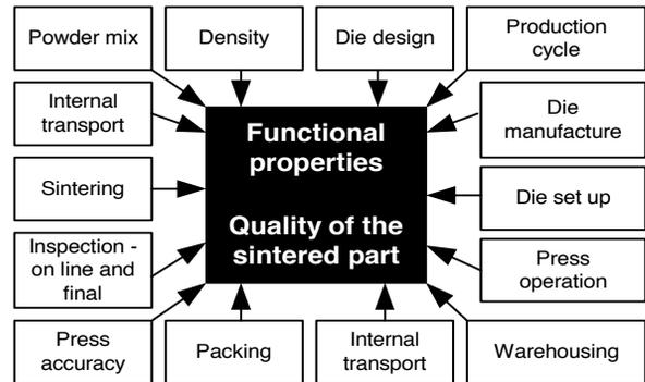
Fig. 2. Parameters controlling the properties of sintered parts and parameters which must be controlled [1]
