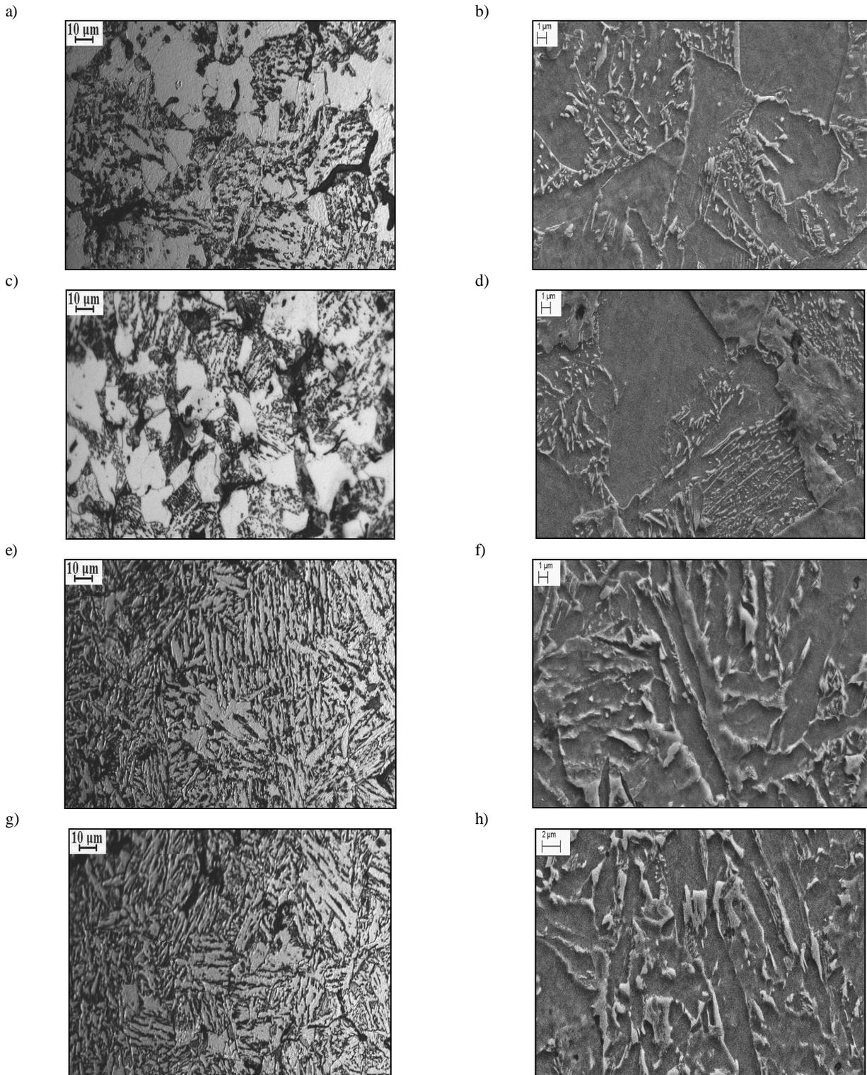
Fig. 9. Microstructure of sintered steels: a,b) Astaloy CrL 500MPa, medium cooling; c,d) Astaloy CrL 600MPa, medium cooling; e, f) Astaloy CrL 500MPa, high cooling; g,h) Astaloy CrL 600MPa, high cooling ; a, c, e, g) light optical microscopy (LOM); b, d, f, h) SEM
