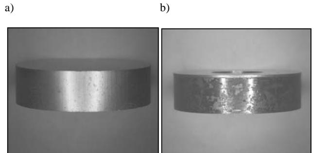
Fig. 14. Example of chosen sample (Astaloy CrL 500MPa, medium cooling) used in wear resistance test; a, b – sample before and after analysis
