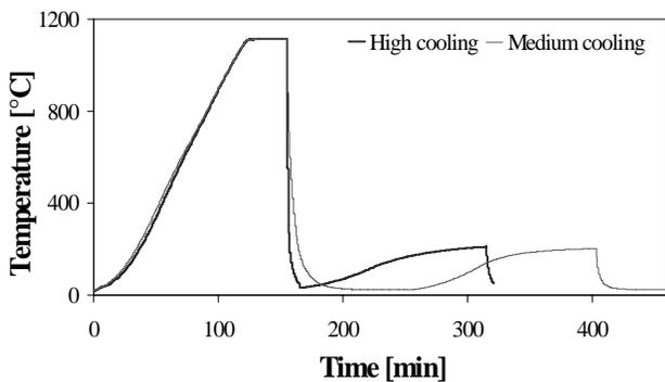
Fig. 4. Samples were sintered and cooled with two different rates and finally tempered
