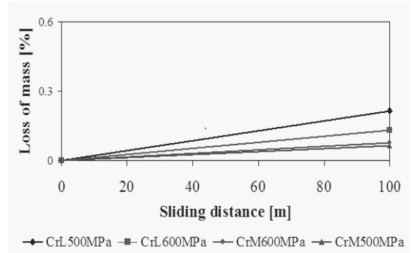
Fig. 12. Loss of mass in a function of sliding distance for the steel cooled with rapid cooling
