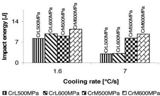
Fig. 11. Charpy impact test performed on materials with medium and rapid cooling
