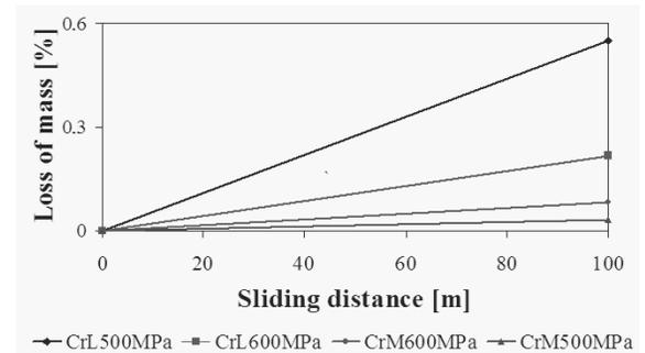
Fig. 13. Loss of mass in a function of sliding distance for the steel cooled with medium cooling
