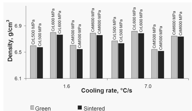
Fig. 5. Green and sintered density of studied compositions (rectangular samples); mean values
