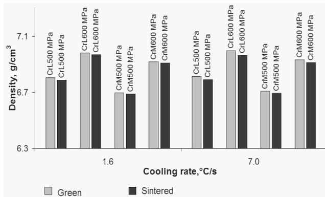
Fig. 6. Green and sintered density of studied compositions (disc samples); mean values
