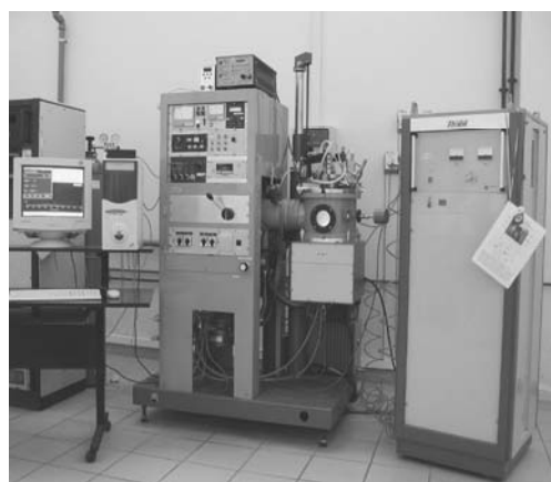
Fig. 1. View of PACVD/MS system
