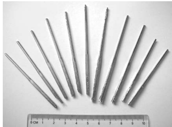
Fig. 1. Outer morphology of cast glassy \text{Fe}_{72}\text{B}_{20}\text{Si}_4\text{Nb}_4 alloy rods with diameters of 1.5 and 2 mm
