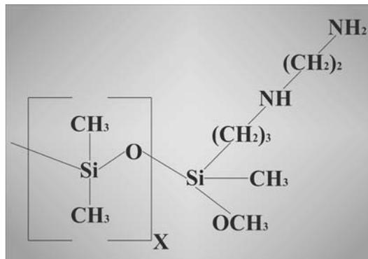
Fig. 4. The diagram of the Dow Corning silicone structure MDX4-4159, 50% Medical Grade Dispersion
