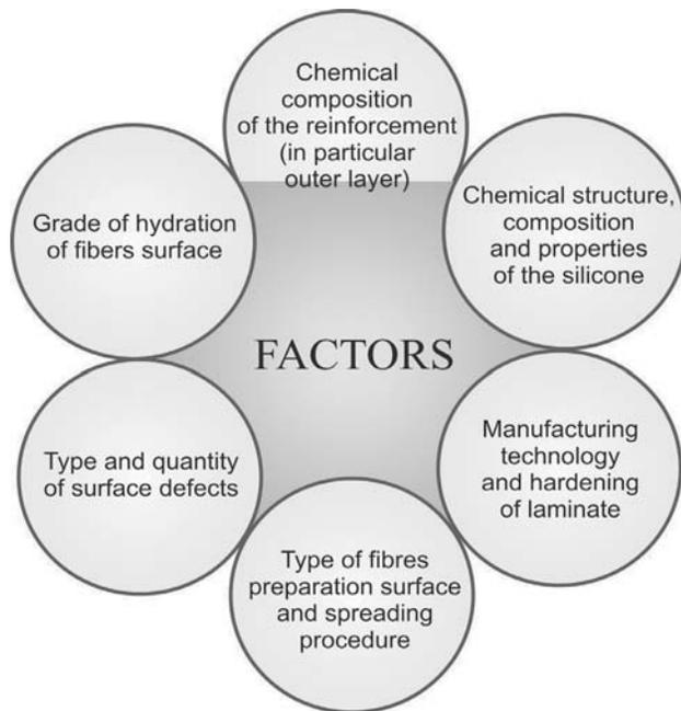
Fig. 6. Factors influencing relations that occur in the interface of the components [16]
