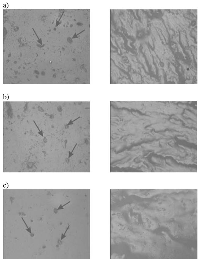
Fig. 10. Surface of samples made based on aramid fabric with basic weight a) 36 g/ m<sup>2</sup>, b) 61 g/m<sup>2</sup>, c) 173 g/m<sup>2</sup>; 40x. Left side – top surface of samples, right side – contact with base bottom surface
