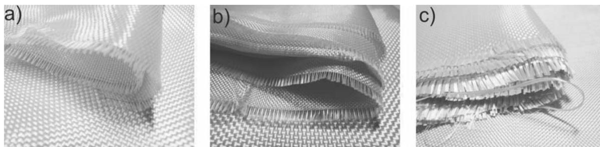
Fig. 3. Aramid fabric with basic weight a) 36g/m<sup>2</sup>; b) 61 g/m<sup>2</sup>; c) 173g/m<sup>2</sup>
