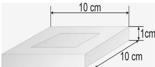
Fig. 9. The demonstrative pattern of the stand for samples
