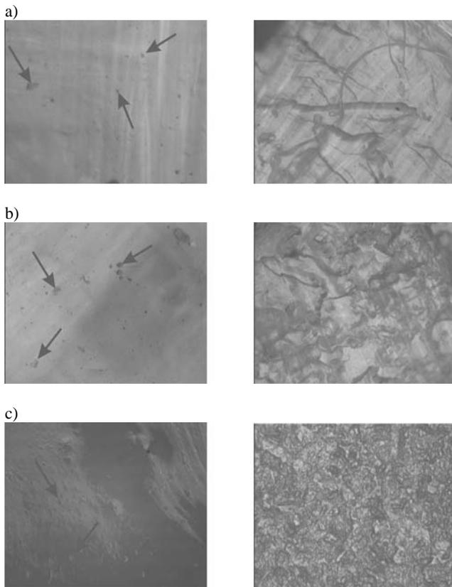
Fig. 11. Surface of samples made based on aramid fabric with basic weight a) 36 g/m<sup>2</sup>, b) 61 g/m<sup>2</sup>, c) 173 g/m<sup>2</sup>(the vacuum chamber); 40x. Left side – top surface of samples, right side – contact with base bottom surface
