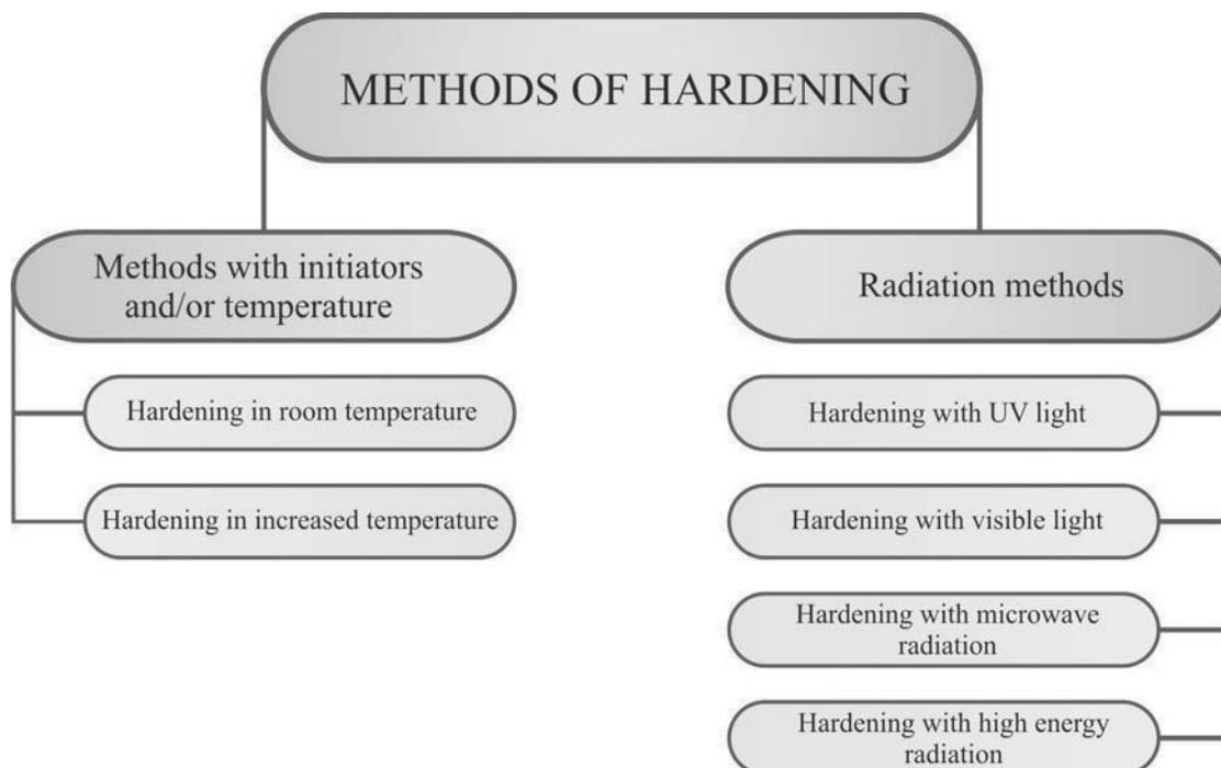
Fig. 7. Division of hardening methods - graphic diagram [6-13]
