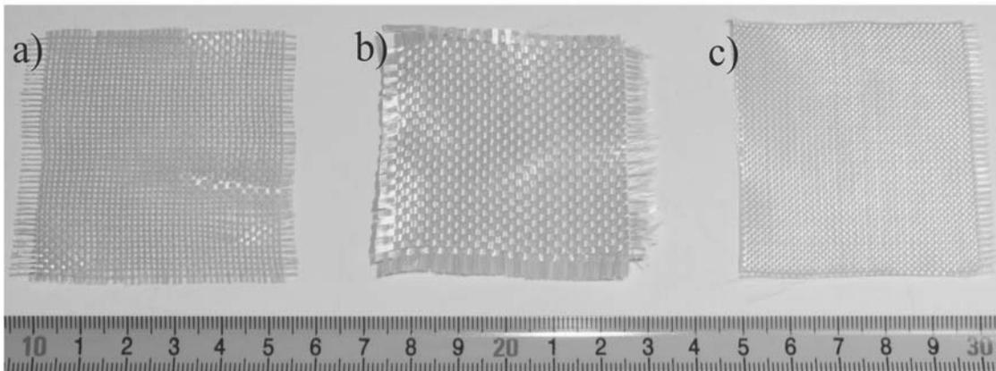
Fig. 8. The survey of prepared samples taken from aramid fabric with basic weight a) 36g/m<sup>2</sup>; b) 61 g/m<sup>2</sup>; c) 173g/m<sup>2</sup>
