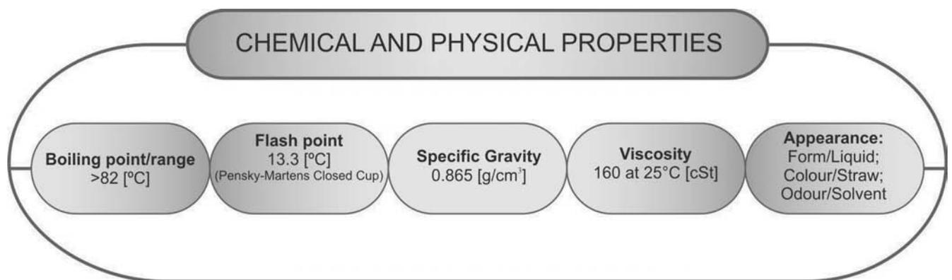
Fig. 5. Chemical and physical properties of medical silicone MDX4-4159 manufactured by COW CORNING
