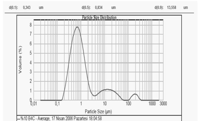
Fig. 4. Particle size distribution of the as-milled C composition
