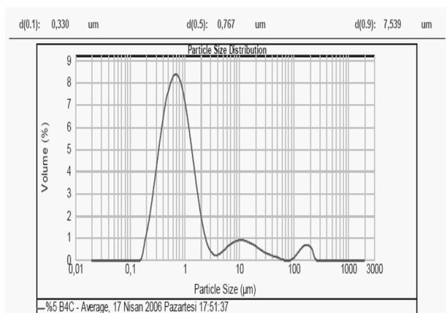
Fig. 3. Particle size distribution of the as-milled B composition
