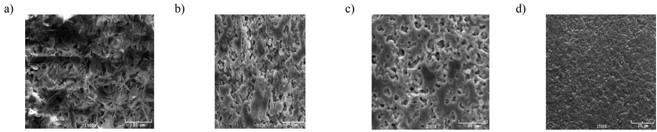
Fig. 7. SEM photographs of different compositions, a) A (100wt% SiC), b) B (95wt% SiC - 5wt% B<sub>4</sub>C), c) C (90wt% SiC - 10wt% B<sub>4</sub>C), d) D (85wt% SiC - 15wt% B<sub>4</sub>C)
