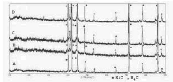
Fig. 6. XRD diffraction patterns of sintered samples
