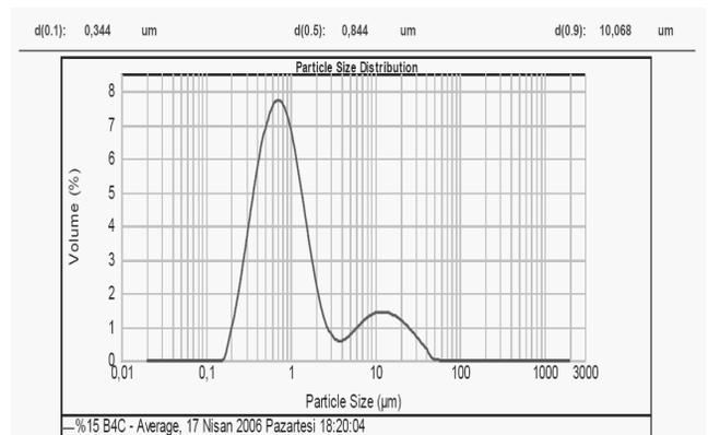
Fig. 5. Particle size distribution of the as-milled D composition
