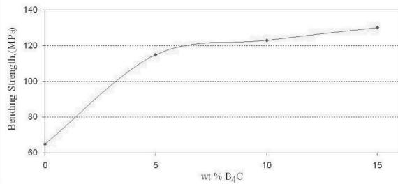
Fig. 8. Relationship between bending strength and % wt B<sub>4</sub>C amount
