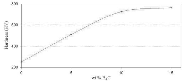
Fig. 9. Vickers hardness versus % wt B<sub>4</sub>C content for different sintered compositions of the present investigation
