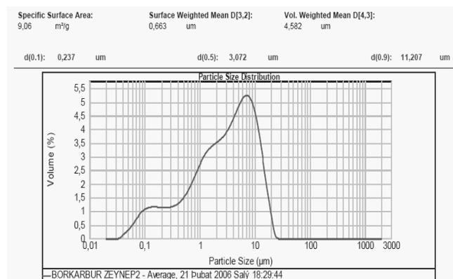
Fig. 2. Particle size distribution of  $B_4C$  powder
