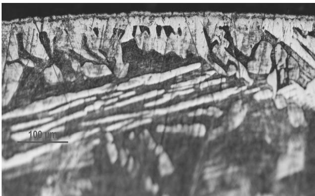
Fig. 1. Optical micrograph of the cross-section of ion-nitrided Ti-6Al-4V samples (x200 magnification)
