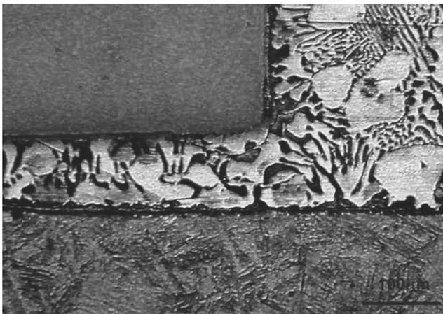
Fig. 8. Brazed joint of X5CrNiMoCuNb14-5 – Ag401 – HF10
