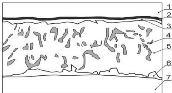
Fig. 13. Scheme of structure brazed joints FerroTitanit Nicro 128 –steel brazed AWS BNi2 filler metal: 1-cermet FerroTitanit Nicro 128, 2- Ni diffusion barrier, 3- transient zone contained cermet and filler metal constituents, 4- intermetallic phase Cr rich, 5- Cr-Fe and Ni solid solution, 6- diffusion zone Cr, Fe and Ni rich, 7- base -steel X5CrNiMoCuNb14-5
