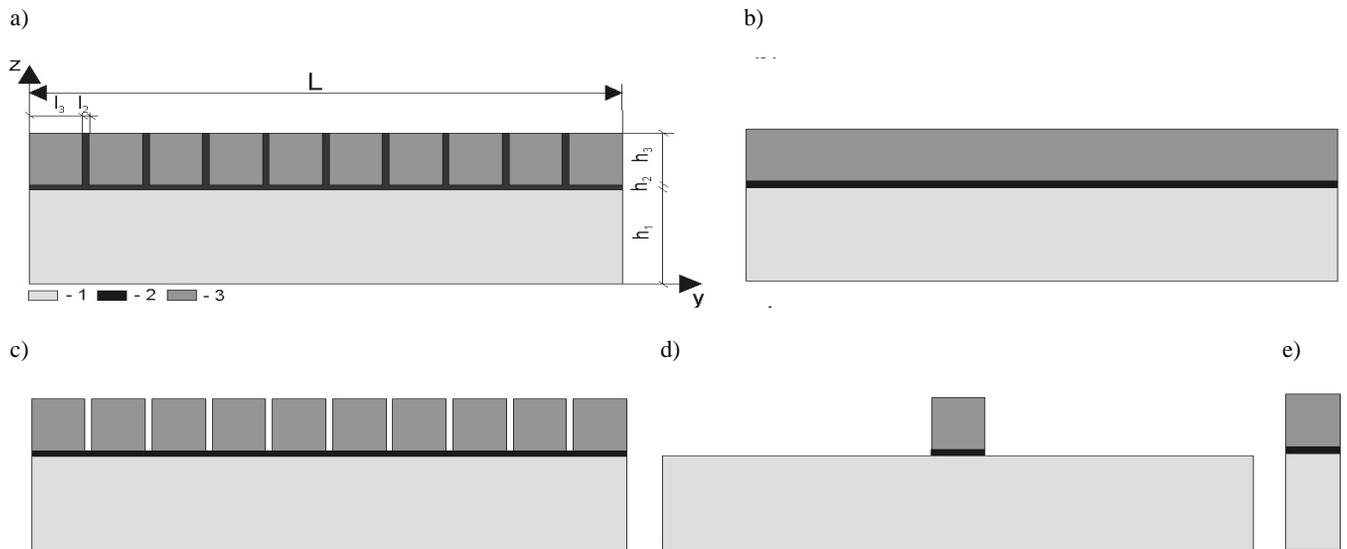
Fig. 15. Two-dimensional physical models brazed joint: 1- steel, 2- filler metal, 3- cermet ( $L=66,35\text{mm}$ ;  $h_1=15\text{mm}$ ;  $h_2=0,15\text{ mm}$ ;  $h_3=8,0\text{ mm}$ ;  $l_2=0,15\text{ mm}$ ;  $l_3 = 6,5\text{ mm}$ ); ten cermet plates, b) one cermet tip about dimension  $L$ , c) ten cermet plates, no vertical gaps, d and e) one cermet plate about dimensional  $l_3$  for small and large steel surface
