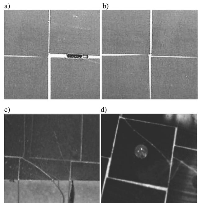
Fig. 4. Examples of defect of the abrasion-resisting layer covered with plates of cermets brazed to the base, a – non-uniform and insufficient thickness of the filler metal between carbides, b – areas unfilled with the filler metal, c and d – cracks of cermet plates as a result of too small seal thickness
