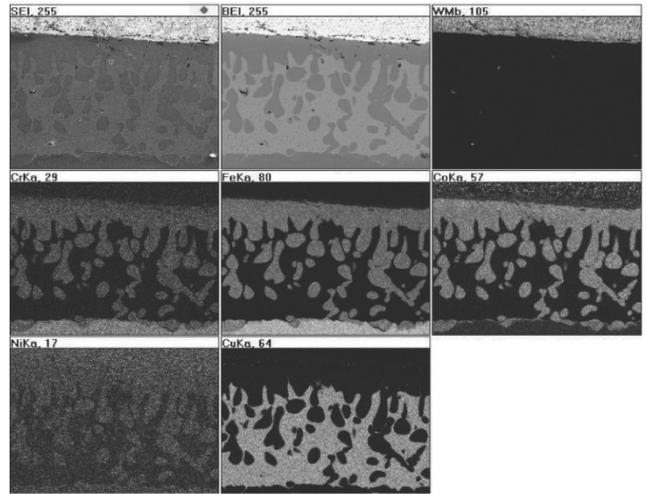
Fig. 9. Brazed joint of X5CrNiMoCuNb14-5 – Cu 106 – G30, chemical distributions of alloying elements
