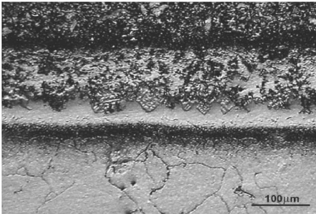
Fig. 7. Microstructure of brazed joint of X5CrNiMoCuNb14-5 – BNi2 – Ferro Titanit Nicro 128
