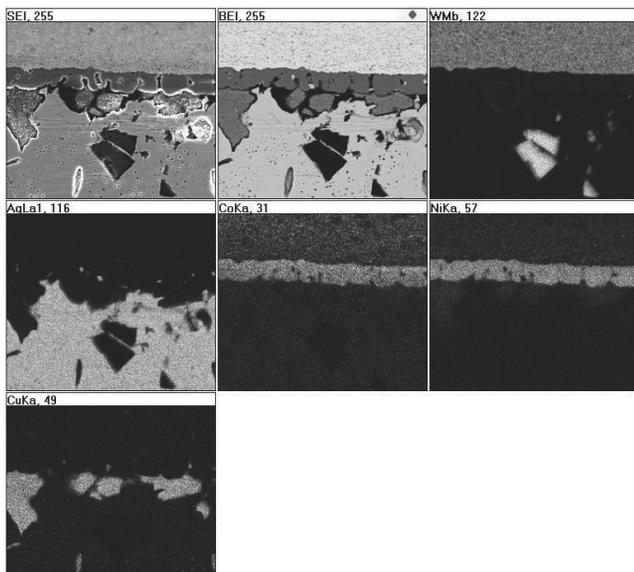
Fig. 11. Brazed joint of X5CrNiMoCuNb14-5 – Ag401 – HF10, chemical distributions of alloying elements
