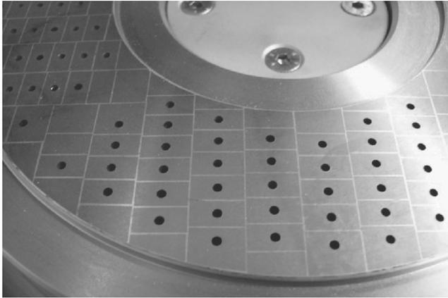
Fig. 3. View of a spinning nozzle used for polyethylene granulation of with the abrasion-resisting layer of a large size surface covered with plates of cermets brazed to the base
