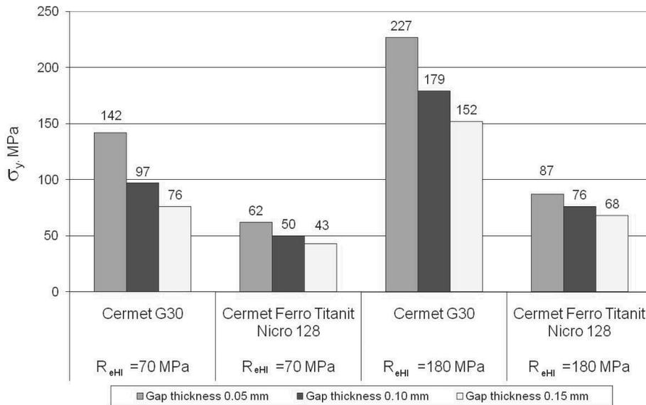
Fig. 16. Comparison of maximum value stresses  $\sigma_y$  for model of different gap thickness, materials and yield stresses, model as on 14a
