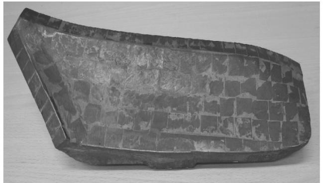
Fig. 2. View of a propeller mixer of ceramic granulated product with the abrasion-resisting layer of a large size surface covered with plates of cermets brazed to the base
