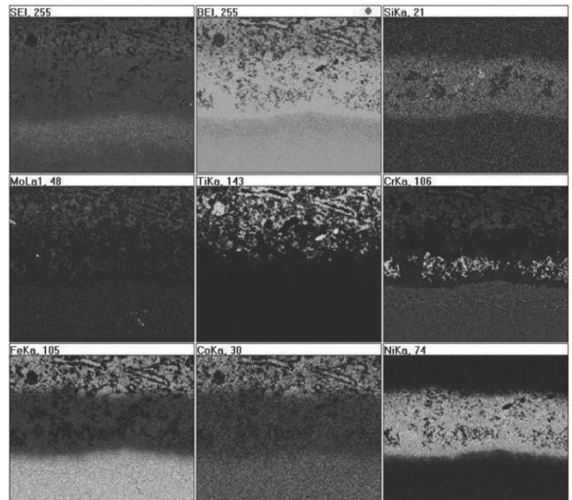
Fig. 10. Brazed joint of X5CrNiMoCuNb14-5 – BNi2 – Ferro Titanit Nicro 128, chemical distributions of alloying elements
