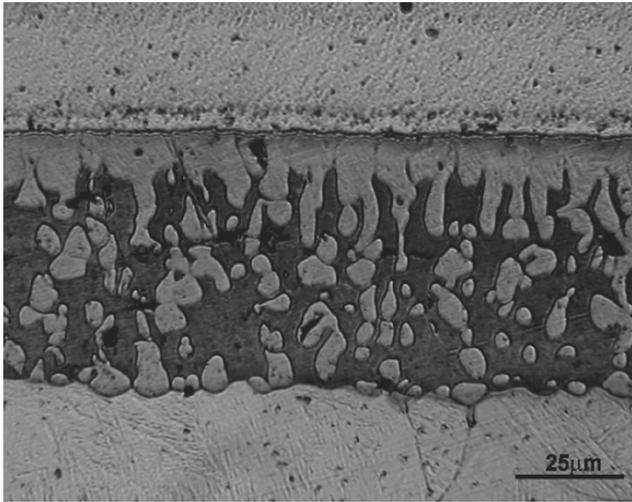
Fig. 6. Brazed joint of X5CrNiMoCuNb14-5 – Cu 106 – G30
