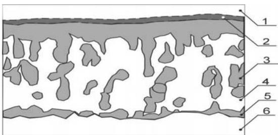
Fig. 12. Scheme of structure brazed joints Cu 106-G30-steel X5CrNiMoCuNb14-5, 1-cermet G30, 2-transient zone contained cermet and filler metal constituents, 3-solder - intermetallic phase from phase equilibrium system Fe-Co, Fe diffusion to steel direction, 4-solder, Cu based solid solution, 5 – transient zone contained steel and filler metal constituents, 6 - steel X5CrNiMoCuNb14-5 base
