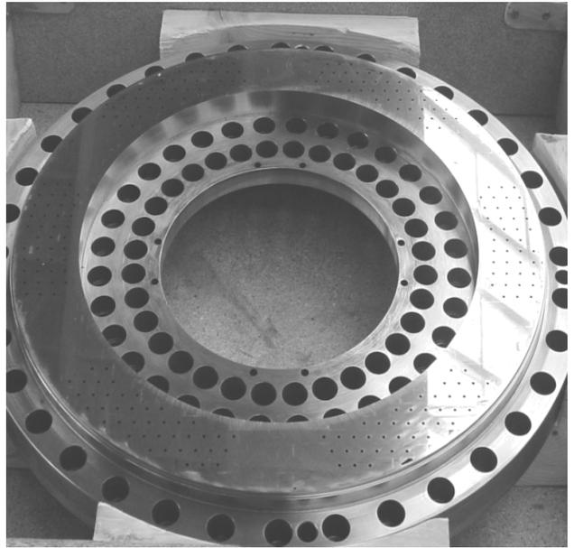
Fig. 1. The view of spinneret for polypropylene granulation with wear resistance layer about high dimensional surface, coated cermet plates
