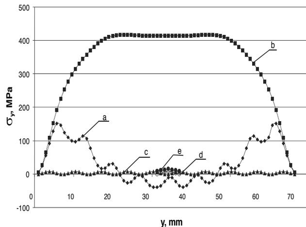
Fig. 17. Normal stresses  $\sigma_y$  in cermet G30 for five models brazed joints, different size of brazing surfaces  $y$ : a) 66,35mm, b) 66,35 mm, c) 66,35 mm, d) 6,5 mm, e) 6,5 mm
