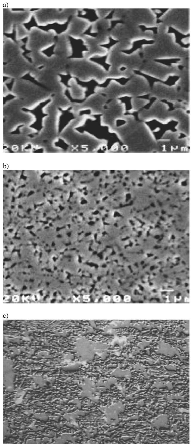
Fig. 5. Microstructure of cermets used of research: a) cermet G30 coarse-grained WC in cobalt matrix, b) submicro cermet HF10, fine-grained WC in cobalt matrix, c) cermet Ferro Titanit Nicro 128 TiC in highly alloyed ferrite matrix
