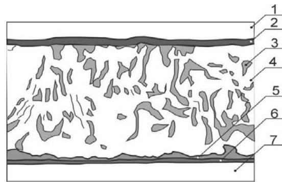
Fig. 14. Scheme of structure brazed joints HF10-AG401 -steel: 1- cermet HF10, 2- transient zone contained cermet and filler metal constituents, 3-solder-intermetallic phase Cu, Ni and Ag, 4 - solder - Ag-Cu solid solution, 5 - transient zone contained steel and filler metal constituents, 6- Ni diffusion barrier, 7 – steel
