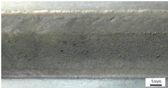
Fig. 28. View of the MCMgAl12Zn1 cast magnesium alloy face weld after laser treatment with WC, scan rate: 0.75 [m/min], laser power: 2.0 [kW]
