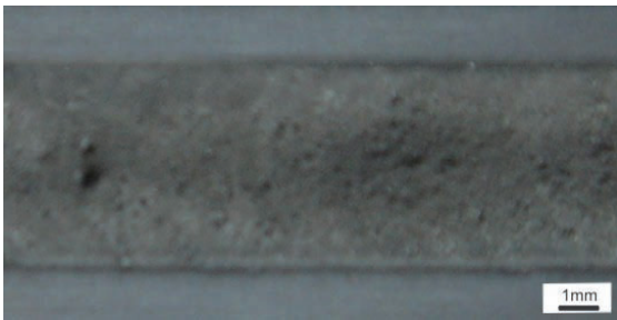
Fig. 29. View of the MCMgAl12Zn1 cast magnesium alloy face of weld after laser treatment with VC, scan rate: 0.75 [m/min], laser power: 1.6 [kW]
