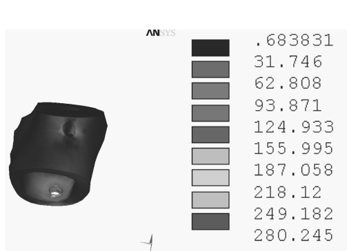
Fig. 10. Stress distribution in a place of a bolt (compression force 1000N), MPa- load step 1, bone model 4
