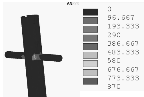
Fig. 18. Stress distribution in a place of a contact between a bolt and intramedullary nail (torsional angel 20°), MPa - load step 2 bone model 4
