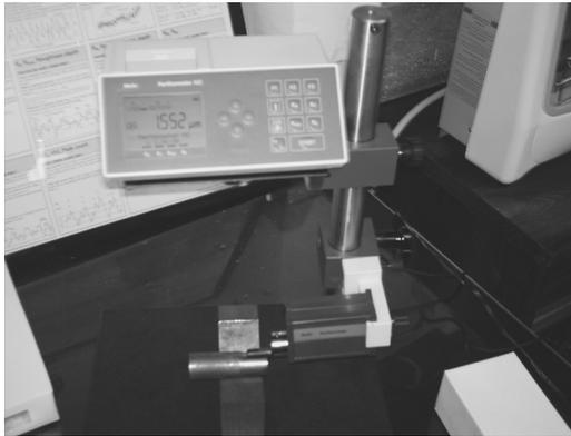
Fig.4. Schematic view of testing perthometer
