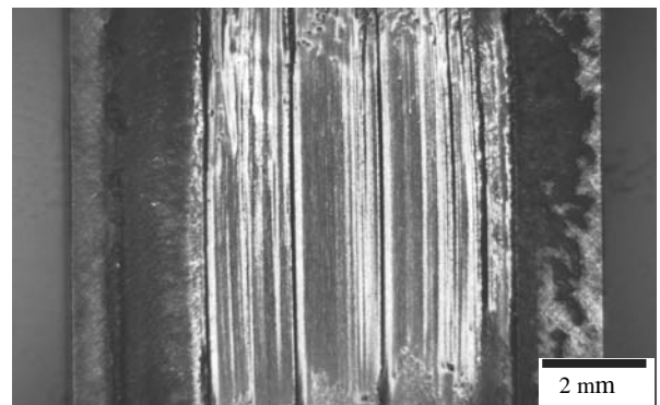
Fig. 10. Surface layer of the test piece from the X40CrMoV5-1 tool steel alloyed TaC, after the wear test, with the following parameters: feed rate-0.5 m/min, the power range 2 kW
