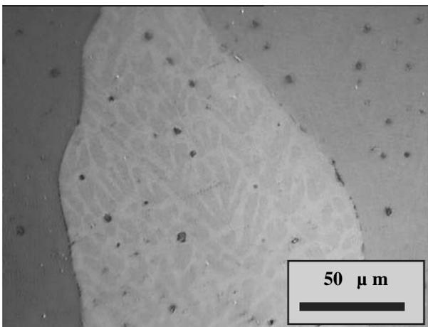
Fig. 11. Microstructure of the  $\text{Al}_2\text{Ti}_2\text{Ce}_2$  alloy in as-cast state
