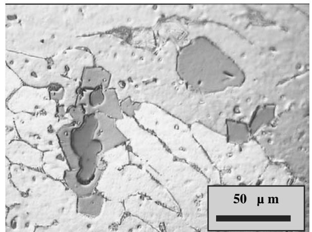
Fig. 14. Microstructure of the Al<sub>2</sub>Ti<sub>2</sub>Ce<sub>4</sub> in as-cast state
