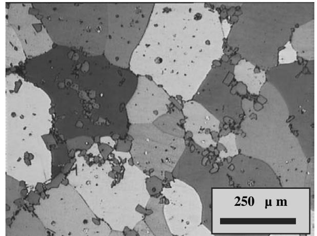
Fig. 13. Microstructure of the Al<sub>2</sub>Ti<sub>2</sub>Ce<sub>4</sub> SHT in 600°C for 4 h
