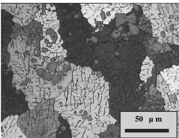
Fig. 12. Microstructure of the Al<sub>2</sub>Ti<sub>2</sub>Ce<sub>4</sub> in as-cast state
