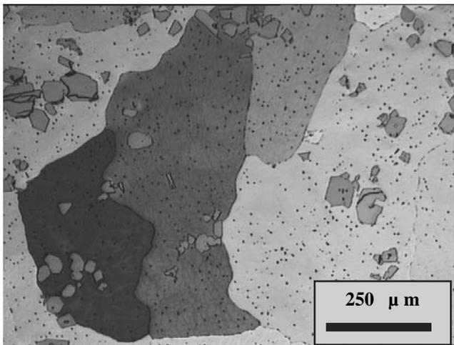
Fig. 8. Microstructure of the Al<sub>2</sub>Ti<sub>2</sub>Ce<sub>2</sub> alloy in the as-cast state
