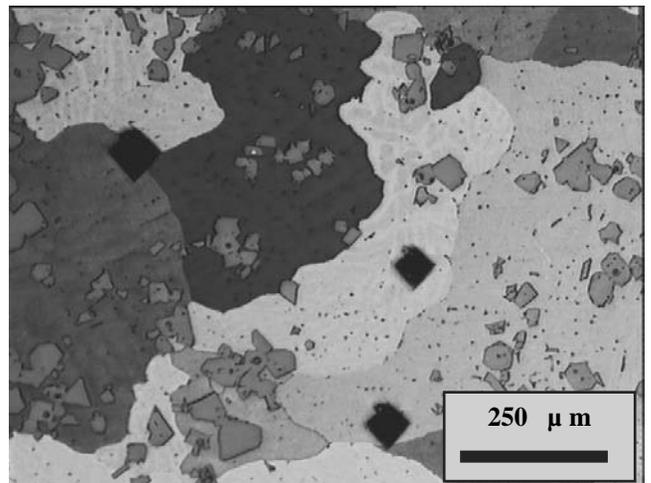
Fig. 9. Microstructure of the Al<sub>2</sub>Ti<sub>2</sub>Ce<sub>2</sub> alloy after SHT in 595 °C for 4 h
