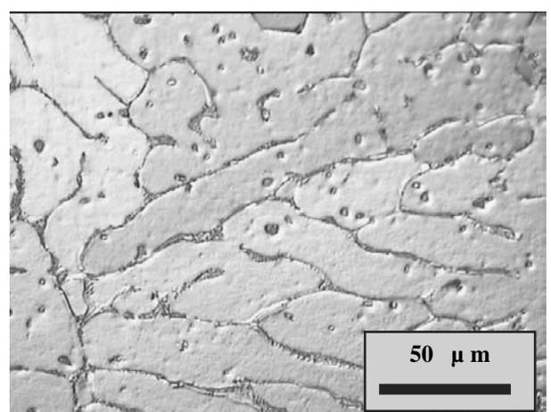
Fig. 15. Microstructure of the Al<sub>2</sub>Ti<sub>2</sub>Ce<sub>4</sub> as-cast
