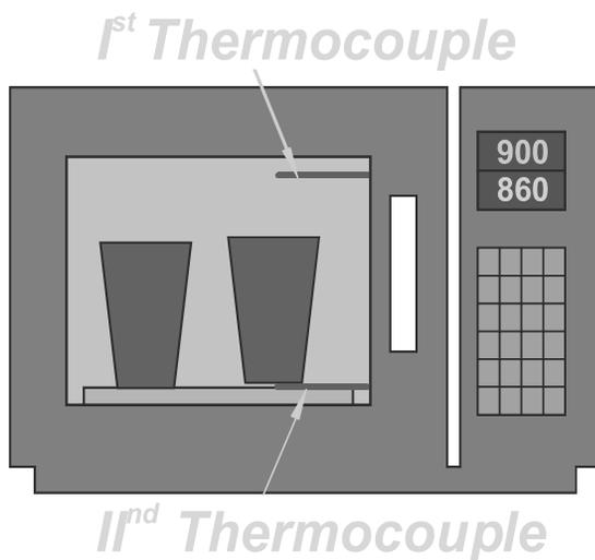
Fig. 2. Schematic thermocouple placement in the electro-resistance furnace
