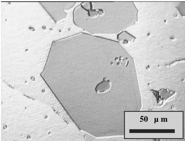
Fig. 10. Microstructure of the Al<sub>2</sub>Ti<sub>2</sub>Ce<sub>2</sub> alloy in as-cast state
