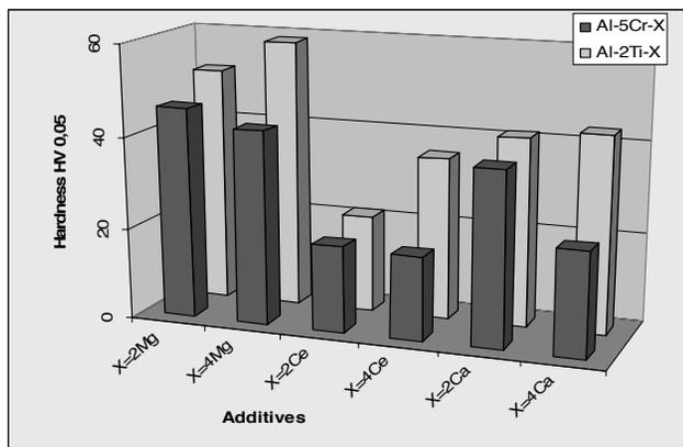
Fig. 16. Hardness measurements results of the alloys with magnesium cerium and calcium addition
