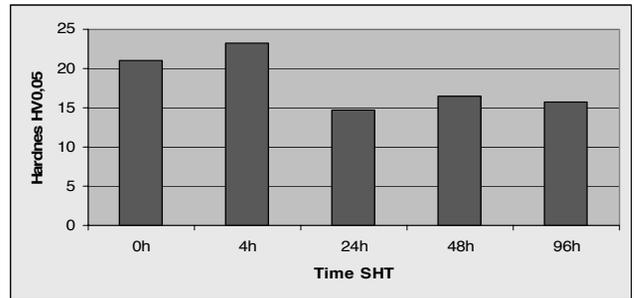
Fig. 5 Hardness measurement results after different times of solution heat treatment
