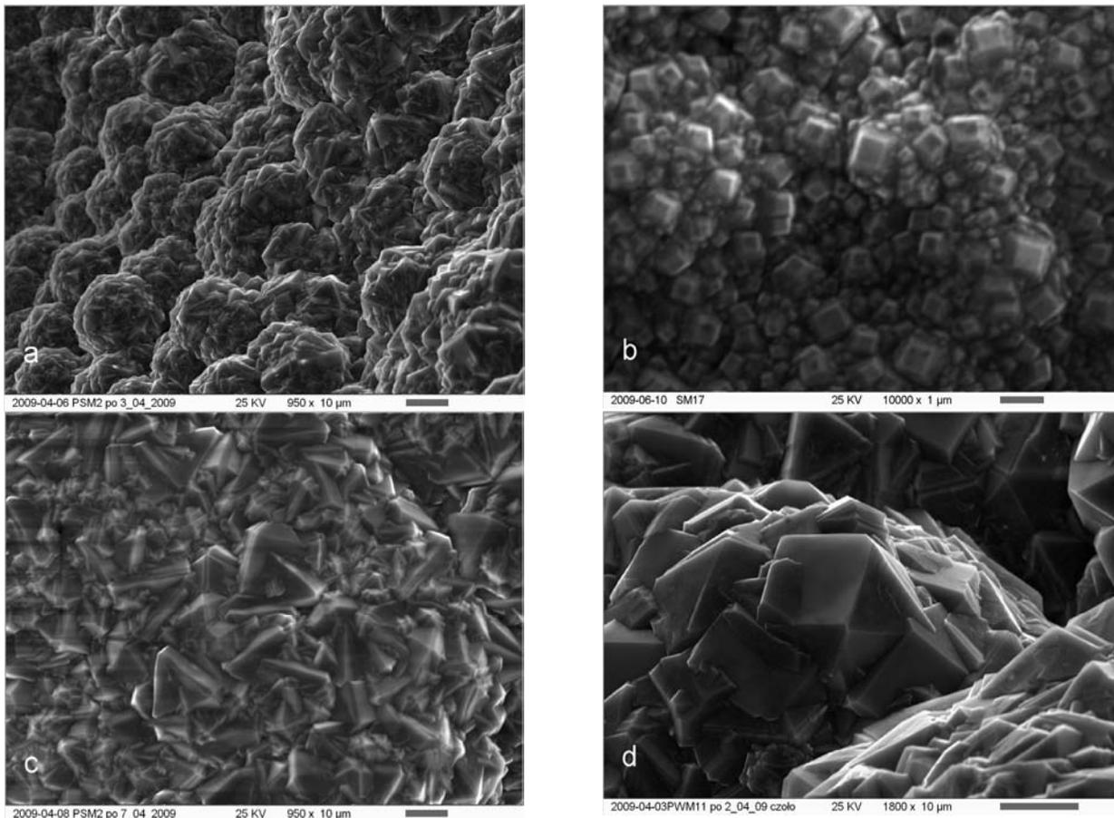
Fig. 1. SEM pictures of diamond layers deposited by HF CVD method
