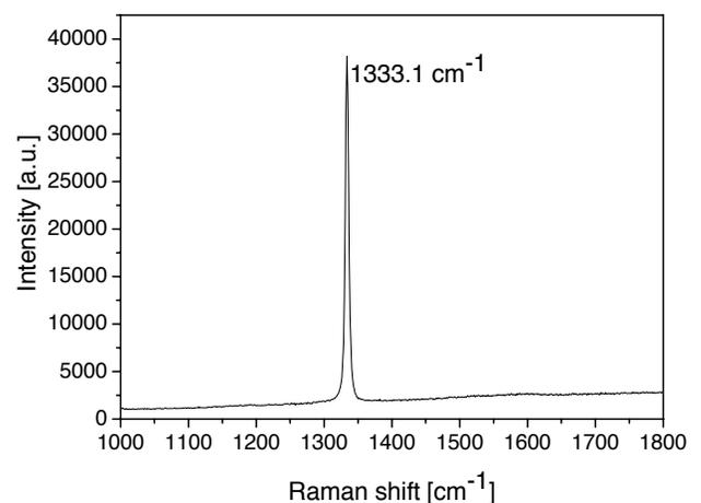
Fig. 3. Raman spectra of the diamond layers from Fig. 1a and Fig. 1d respectively
