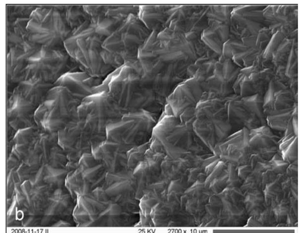
Fig. 4. SEM image of working electrode head covered with diamond films: (a) general view, (b) details of diamond film morphology
