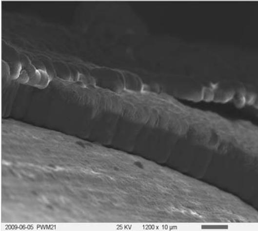
Fig. 2. Cross section of polycrystalline diamond film
