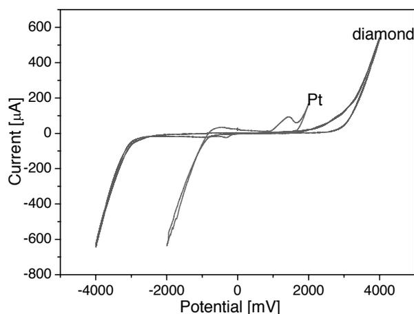
Fig. 5. Cyclic voltammograms registered by Pt and diamond electrodes in 0.025M NaCl at a scan rate of 200 mV/s
